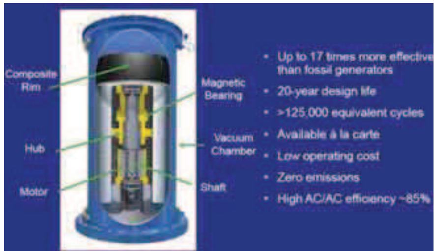
Fig. 7. Flywheel technology of Beacon POWER [8]
