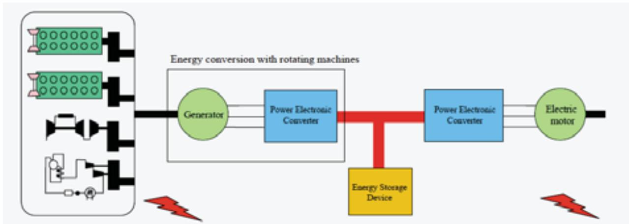
Fig. 1. Structure of combined ship's power plant [1]
