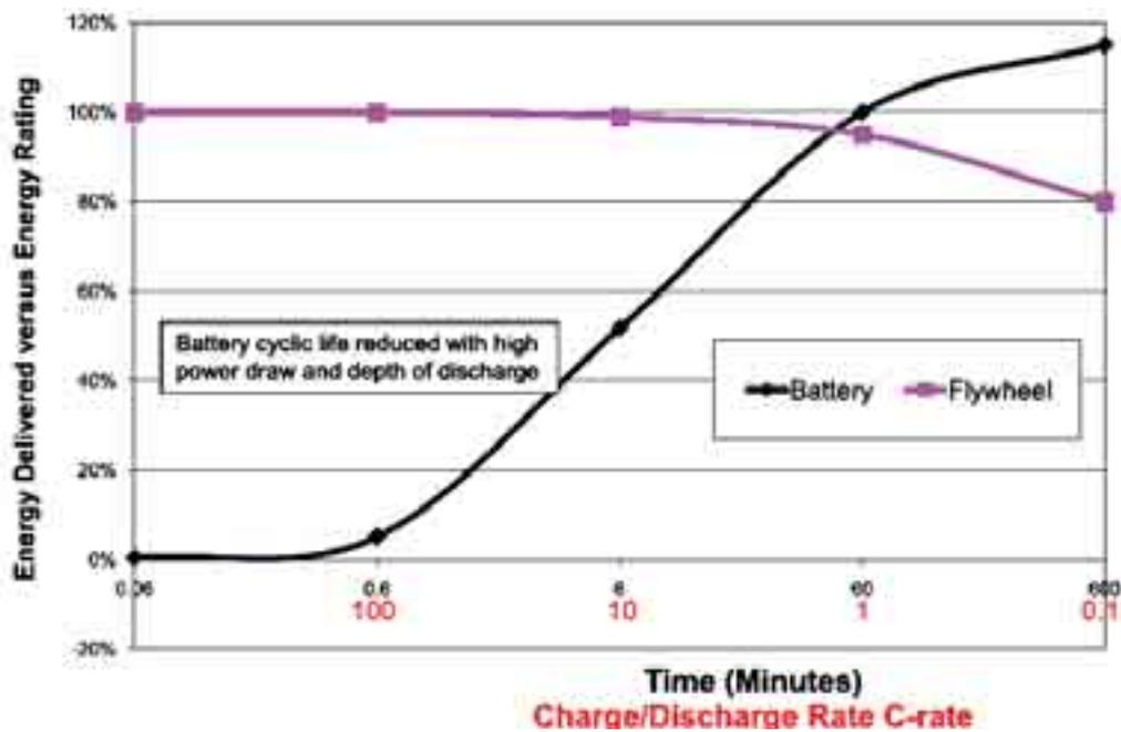
Fig. 6. Energy delivered versus energy rating for battery and flywheel [8]
