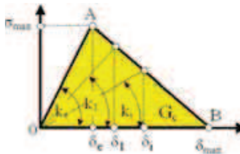
Fig. 5. Bi-linear cohesive element. There are five available parameters to define the element. They are k_e , G_c , \sigma_{max} , \delta_x and \delta_{max} . However only three are independent
