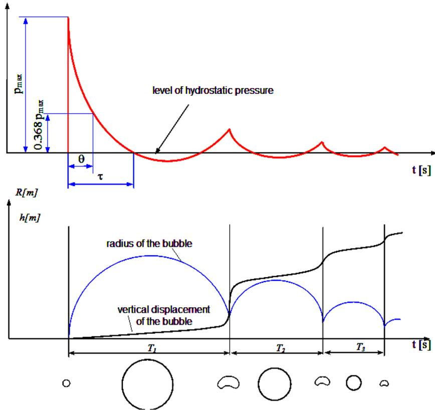
Fig. 1. Gas bubble pulsations during an underwater explosion [3]
