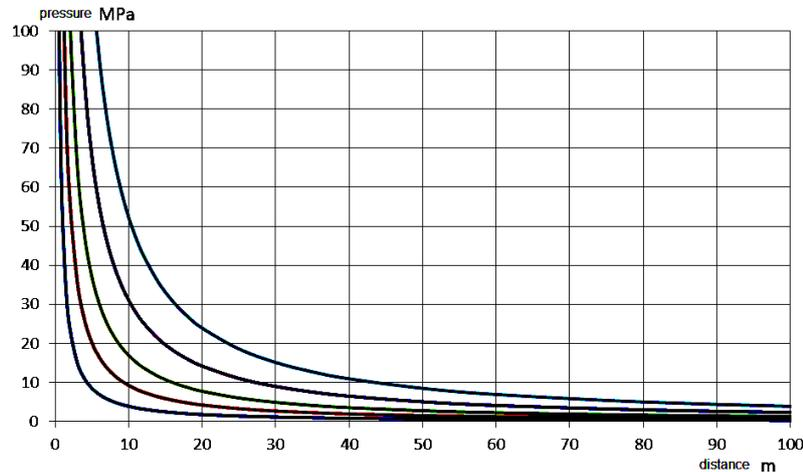
Fig. 10. Pressure values at the front of the shock wave as a function of load mass of TNT of 1, 10, 50, 250, 1000 kg
