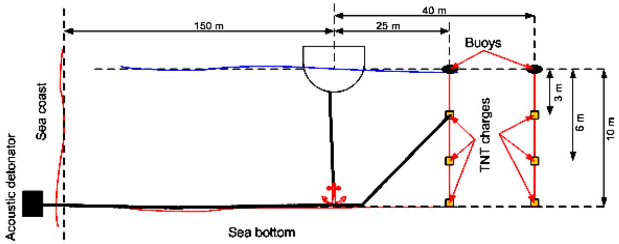
Fig. 3. Distance and depth of TNT charges placement
