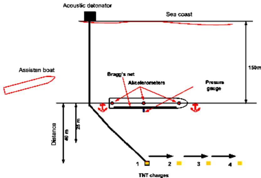
Fig. 2. Schematic layout of underwater detonation experiments.
