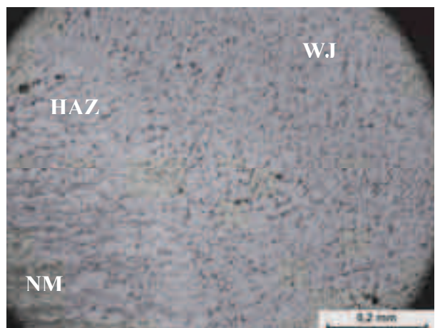
Fig. 4. Microstructure of joints: a) welded by FSW, b) welded by MIG
