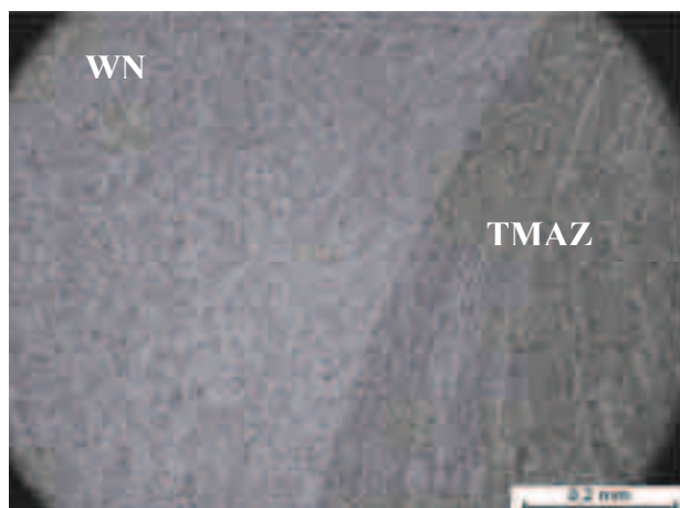
Fig. 4. Microstructure of joints: a) welded by FSW, b) welded by MIG
