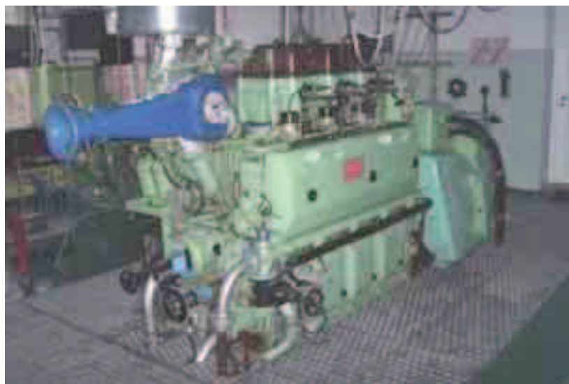
Fig. 1. General view of the Sulzer 3 AL 25/30
