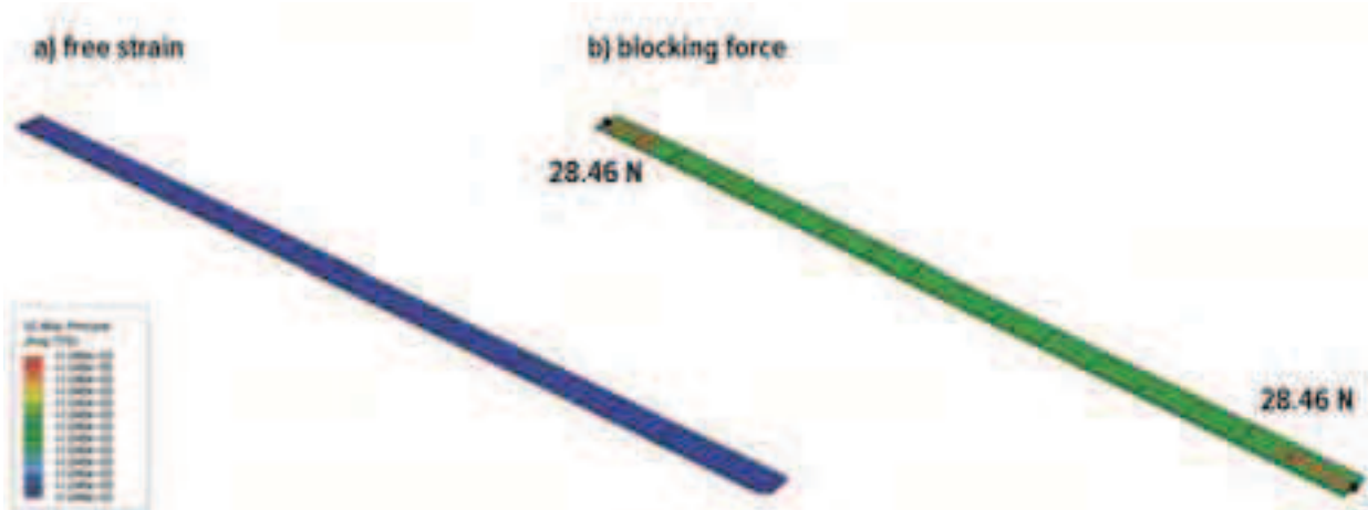
Fig. 2. Numerical tests for the separated M-8503-P1 piezoelement: a) free strain extension, b) blocking force
