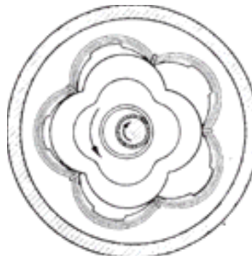
Fig. 5. Geometry of rotary piston and motionless cylinder of RENAULT-AMERICAN MOTORS [1]
