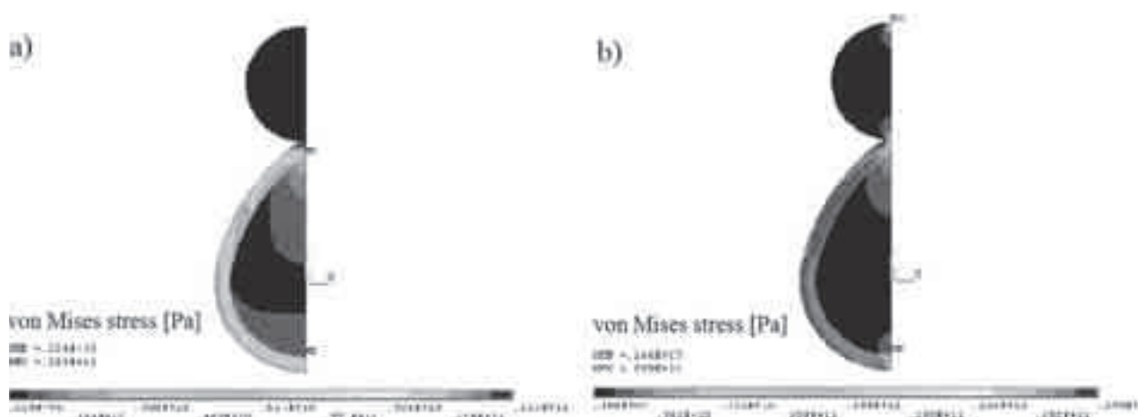
Fig. 8. von Mises stresses for angular position \alpha = 0^\circ for roller of tappet in respect to camshaft axis; a) the first load case, b) the second load case
