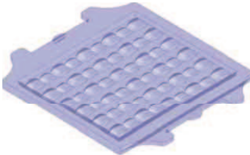
Fig. 1. A considered pad with cylindrical-shaped elements in its working area [2]
