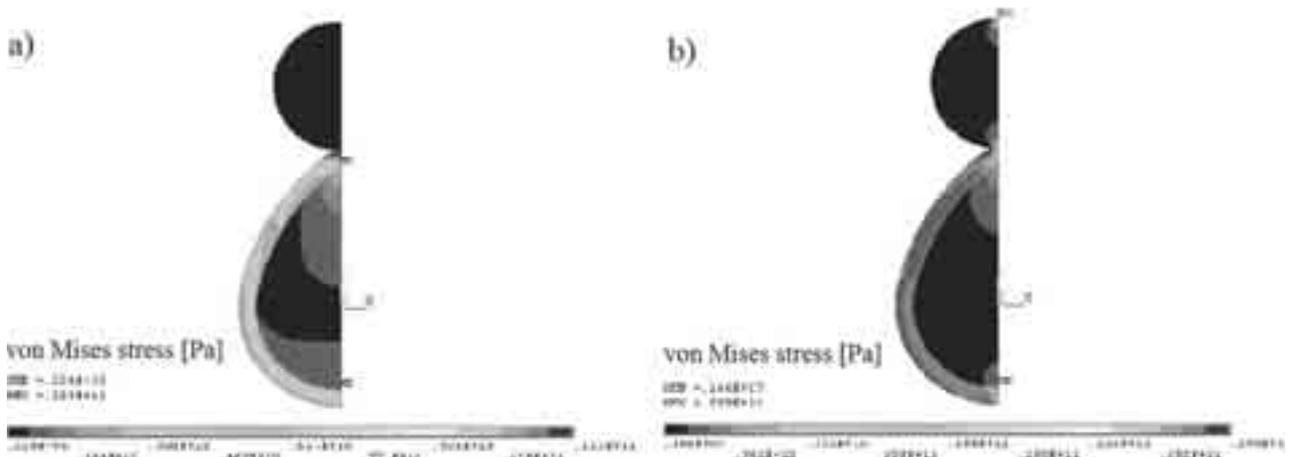
Fig. 8. von Mises stresses for angular position  $\alpha = 0^\circ$  for roller of tappet in respect to camshaft axis; a) the first load case, b) the second load case
