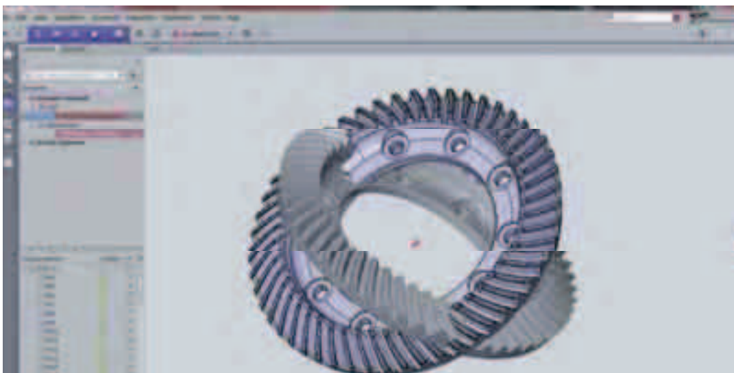
Fig. 4. Combining nominal model of the 3D-CAD with measure gear
