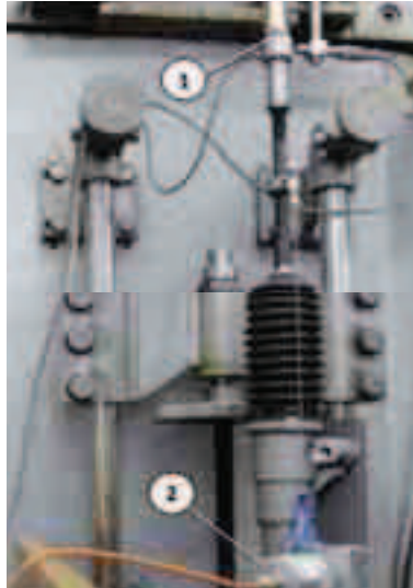
Fig. 7. Input function system; 1 – force sensor; 2 – cable sensor of the toothed bar displacement
