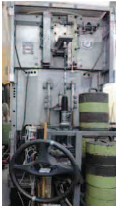
Fig. 6. Measuring stand adapted to input function on the side of the gear-toothed bar. Examined toothed bar is in a vertical position
