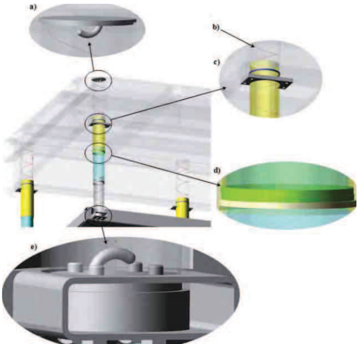
Fig. 3. Construction of telescopic-elastic mechanism of opening the cassette bottom: a) fastening the spring from the side of the roadway, b) spring, c), elements of fastening the upper cylinder, d) assembling the cylinders of telescopic mechanism, e) elements of fastening the spring and lower cylinder with movable bottom of the cassette
