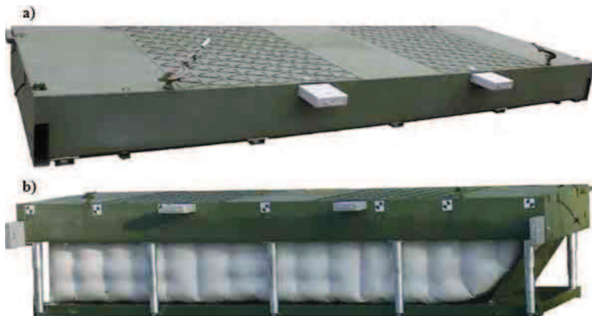
Fig. 1. Prototypical cassette of a floating bridge; a) closed; b) open with lowered bottom and visible pontoon-container filled with the air
