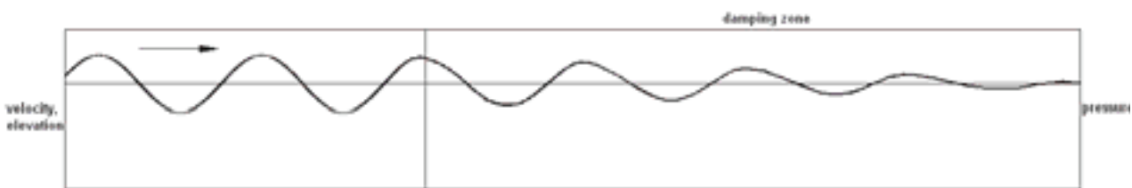
Fig. 2. Generating the waves by prescribed wave motion and suppressing them in the damping zone
