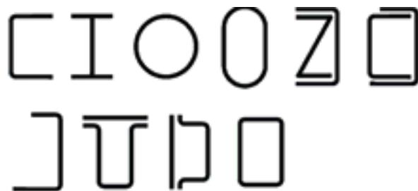
Fig. 2. Typical cross sections of profiles used in frames [5]
