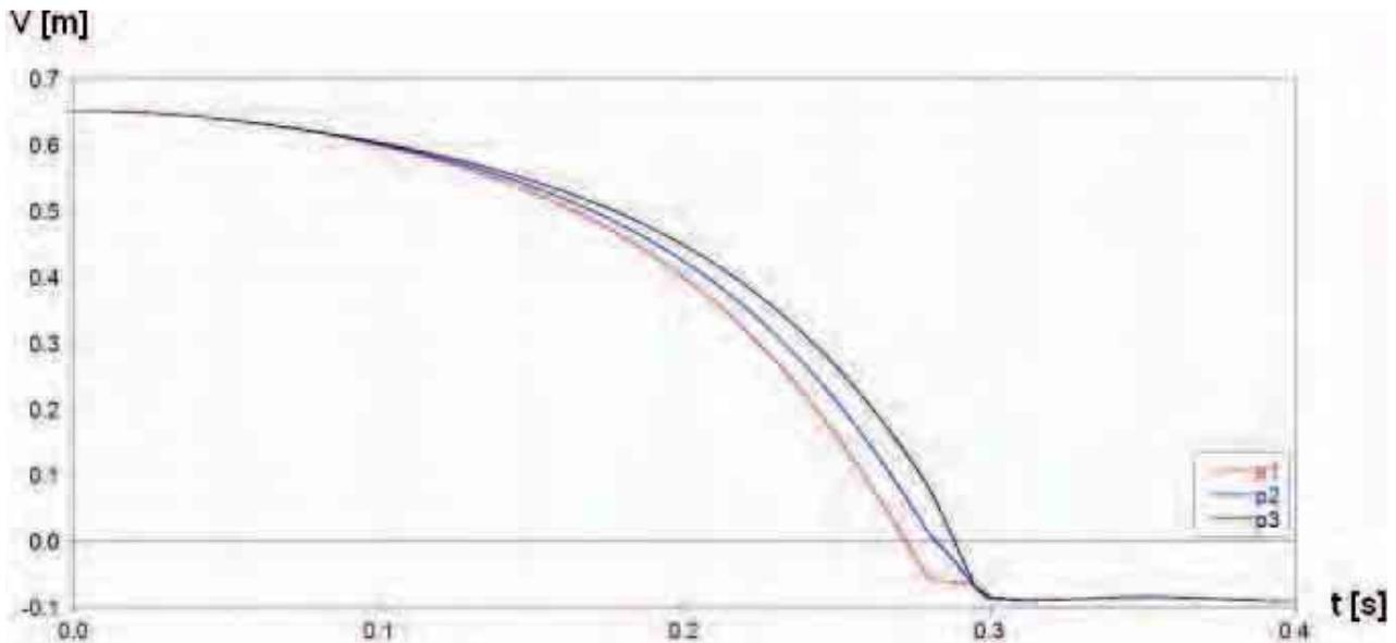
Fig. 6. Displacement of measurement points  $P_1$ ,  $P_2$  and  $P_3$  on the cassette bottom – variant III
