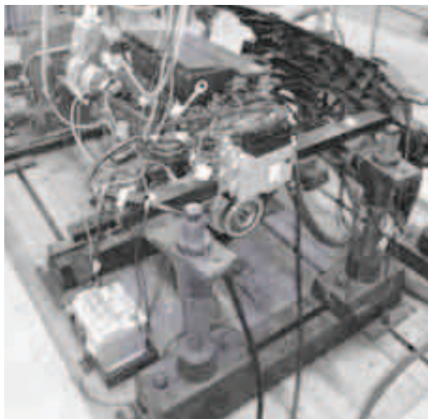
Fig. 3. The view of Fiat 1.3 JTD 16 V Multijet engine connected with eddy current brake EMX 100 by means of drive shaft
