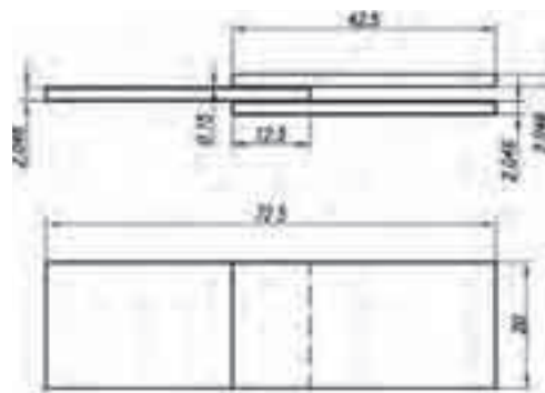
Fig. 2. Functional diagram and the dimension of the steel (S355J2G3) double lap specimen (dimensions in mm)
