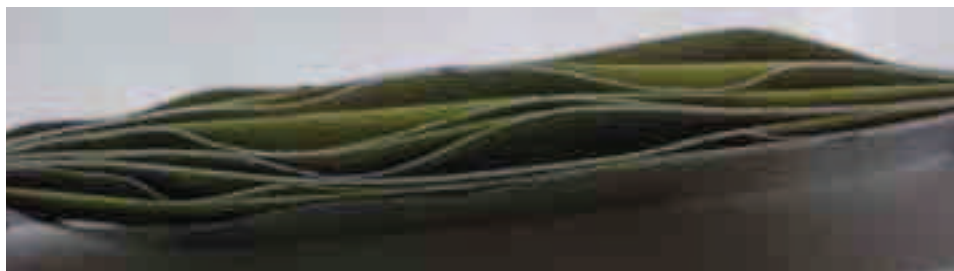
Fig. 14. Delaminated specimen of laminar composite
