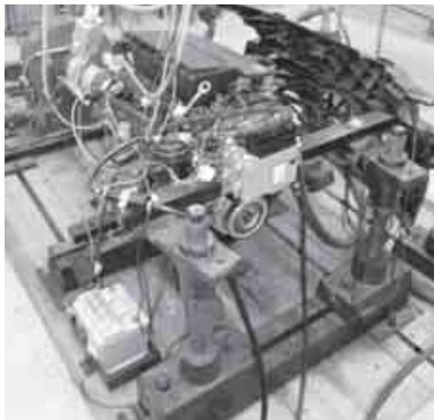
*Fig. 3. The view of Fiat 1.3 JTD 16 V Multijet engine connected with eddy current brake EMX 100 by means of drive shaft*
