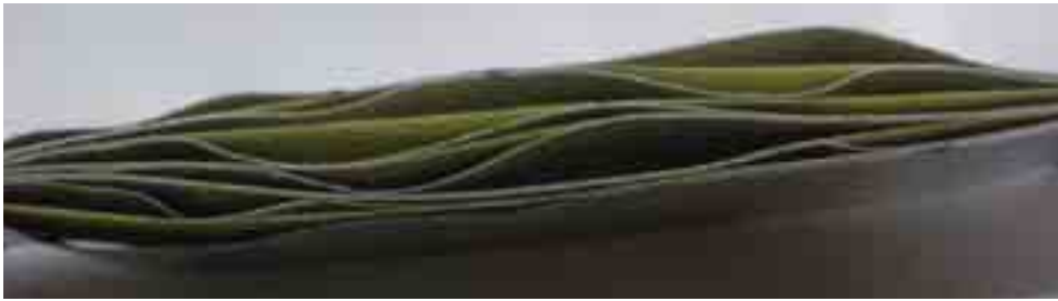
Fig. 14. Delaminated specimen of laminar composite
