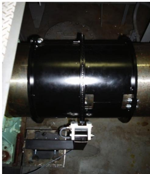
*Phot. 1. Toothed rings and laser sensor mounted at intermediate shaft*
