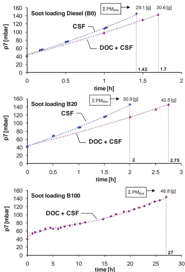
Fig. 2. Backpressure ( $p_7$ ) during soot loading cycle
