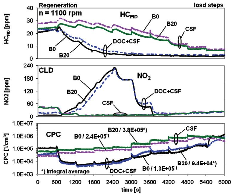
Fig. 5. Regeneration with (DOC + CSF) vs. (CSF) with B0 & B20
