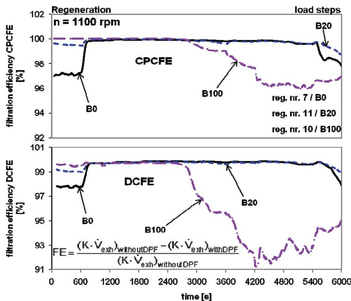
Fig. 4. Instantaneous nanoparticle filtration efficiency during the regeneration procedures with (DOC+CSF) & B0, B20, B100
