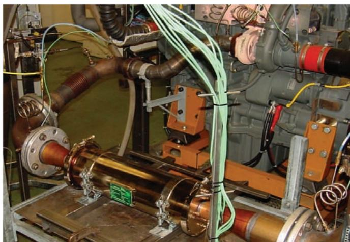
*Fig. 1. HUG DPF with passive regeneration (DOC+CSF) on the Liebherr engine*
