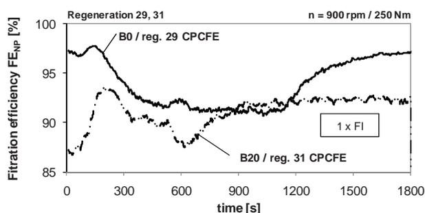
Fig. 9. CPC filtration efficiency during regeneration with B0 & B20
