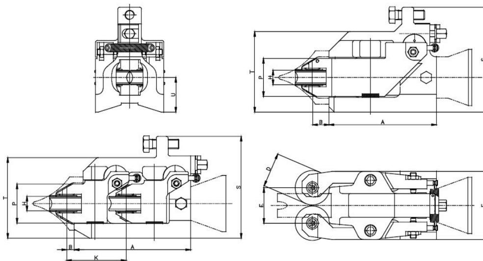
Fig. 14. Entry guide for fast rolling sketch [2]
