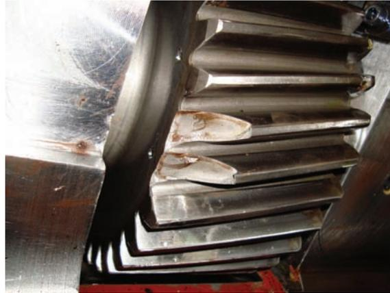
Fig. 3. Broken teeth on the sprocket
