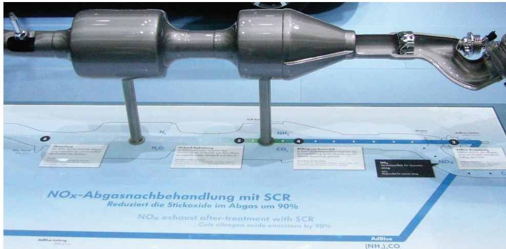
Fig. 4. Reactor SCR of 2.0 TDI engine
