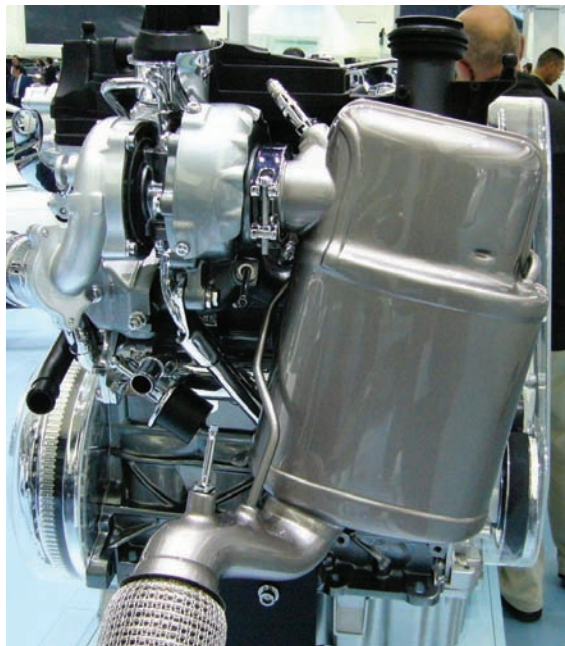
Fig. 3. Standard exhaust gases cleaning module
