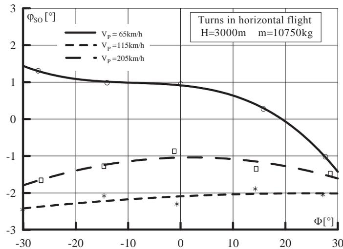
Fig. 8. Relationship between the pitch angle  $\varphi_{SO}$  of the tail rotor and the bank angle  $\Phi$  of the helicopter. The relationships are shown for various values of the flights speed  $V_P$  with turns during horizontal flights
