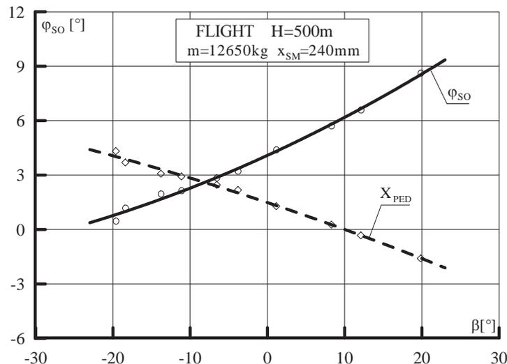
Fig.6. Relationship between the stroke  $\varphi_{SO}$  of the tail rotor and deviation  $X_{PED}$  of pedals versus the  $\beta$  slip angle during the travel phase
