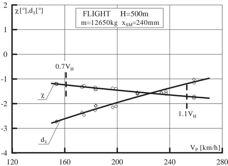
Fig. 5. Relationship between the inclination angle  $\chi$  of the steering disk and leaning  $d\chi$  of the control stick versus the instrumental flight speed  $V_P$  for the travel phase
