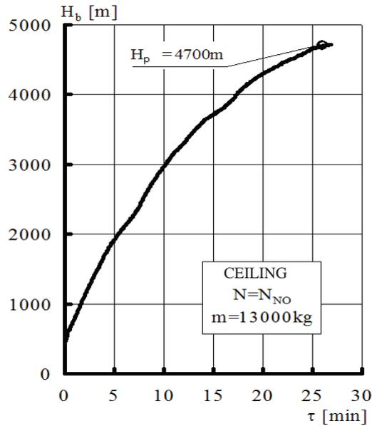
Fig.2. Relationship between the climbing time  $\tau$  and the function of barometric altitude  $H_b$
