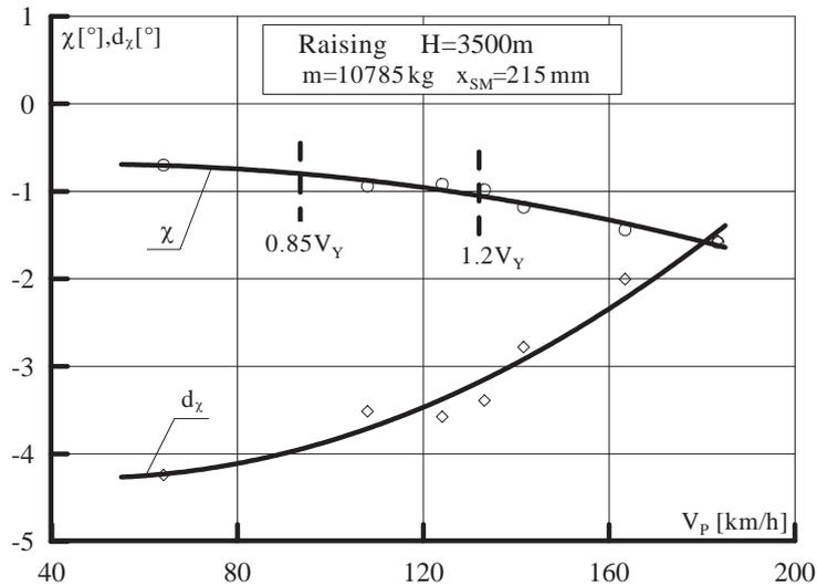
Fig. 4. Relationship between the inclination angle  $\chi$  of the steering disk and leaning  $d\chi$  of the control stick versus the instrumental flight speed  $V_P$  for the ascending phase.
