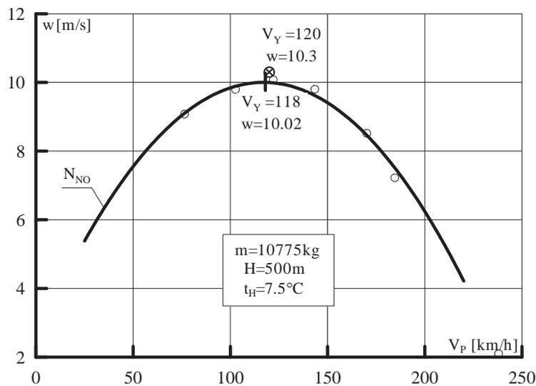
Fig. 1. The relationship between ascending velocities of the aircraft and the instrumental speed values  $V_P$  of flights with the rated power  $N_{NO}$  of the driving unit operation
