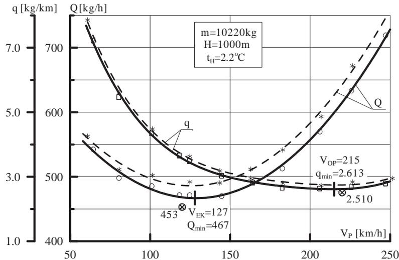
Fig. 3. Relationships between the fuel amount consumed by the helicopter per hour ( $Q$  and per kilometre ( $q$ ) of flight and the speed  $V_P$  of the horizontal flight indicated by the cockpit instruments
