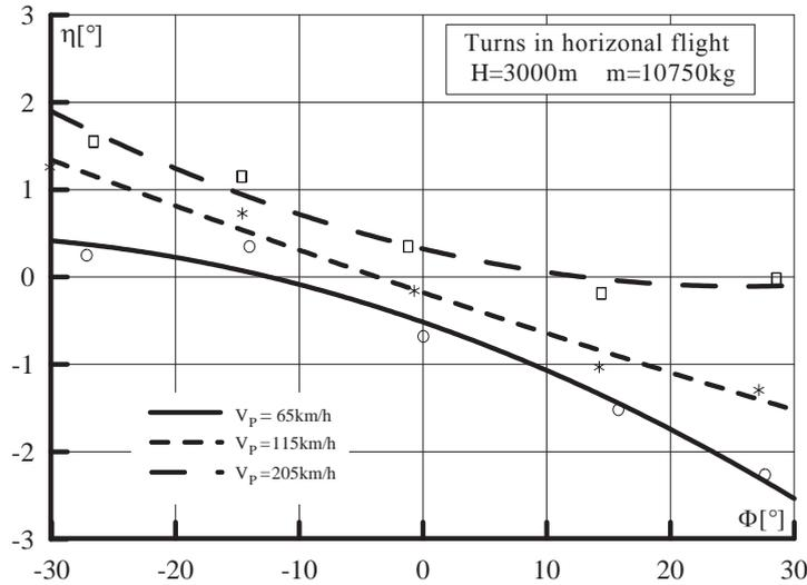
Fig. 7. Relationship between the tilt angle  $\eta$  of the steering disk and the bank angle  $\Phi$  of the helicopter. The relationships are shown for various values of the flights speed  $V_P$  with turns during horizontal flights
