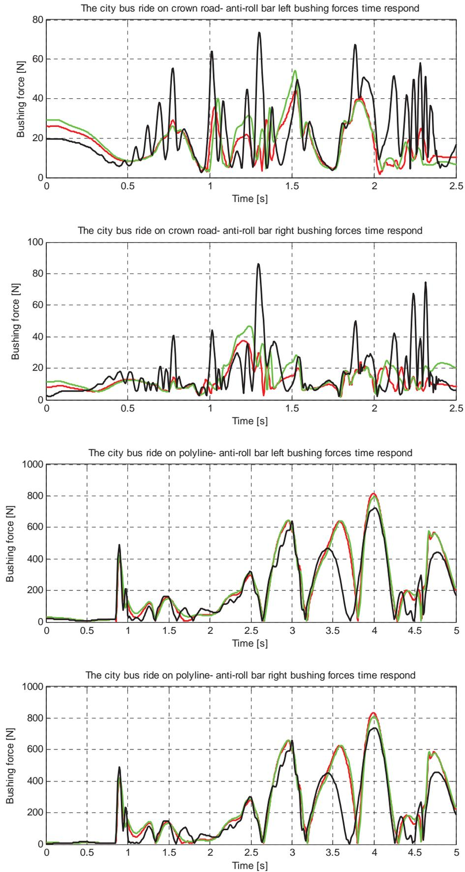
Fig. 6. Anti-roll bar bushing force time respond with tree different force-velocity characteristics of damper element while riding on two different road profiles (crown upper one and polyline lower one)
