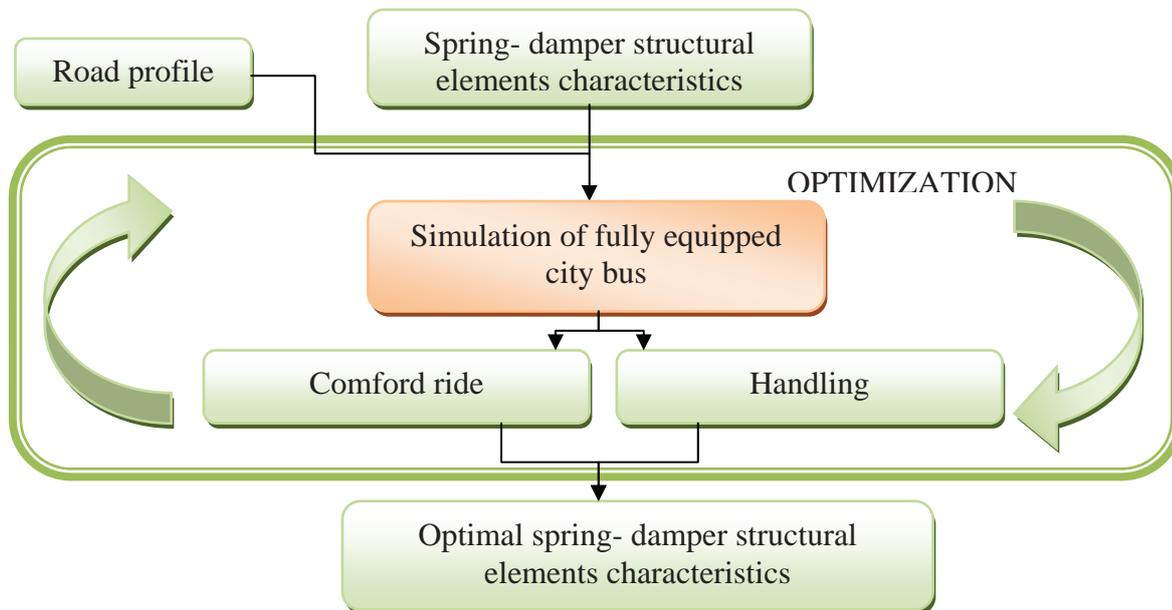
Fig. 8. Schema of multi-objective optimization process using multibody model and simulations
