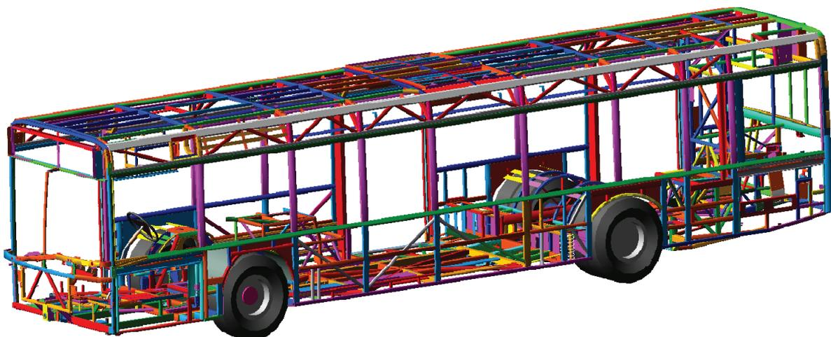
*Fig. 2. The multibody model of the city bus*
