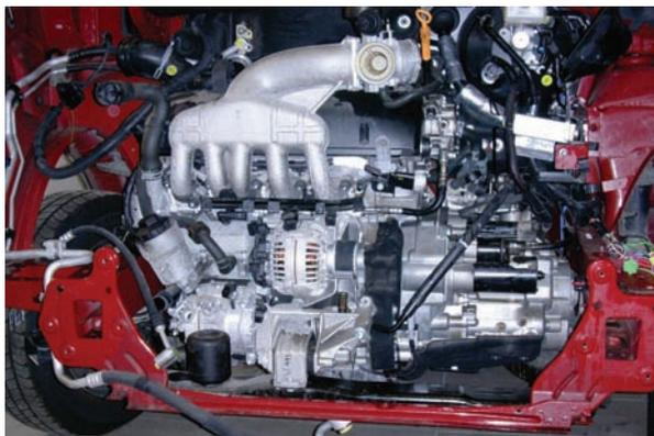
Fig. 1. A 5-cylinder engine of a VW Transporter van
