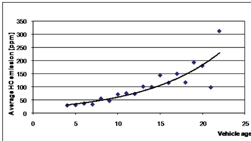
Fig. 10. Average HC emission for a particular vehicle age (2500 rpm)
