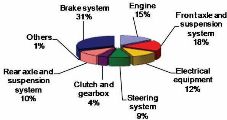
Fig. 2. Structure of vehicle faults
