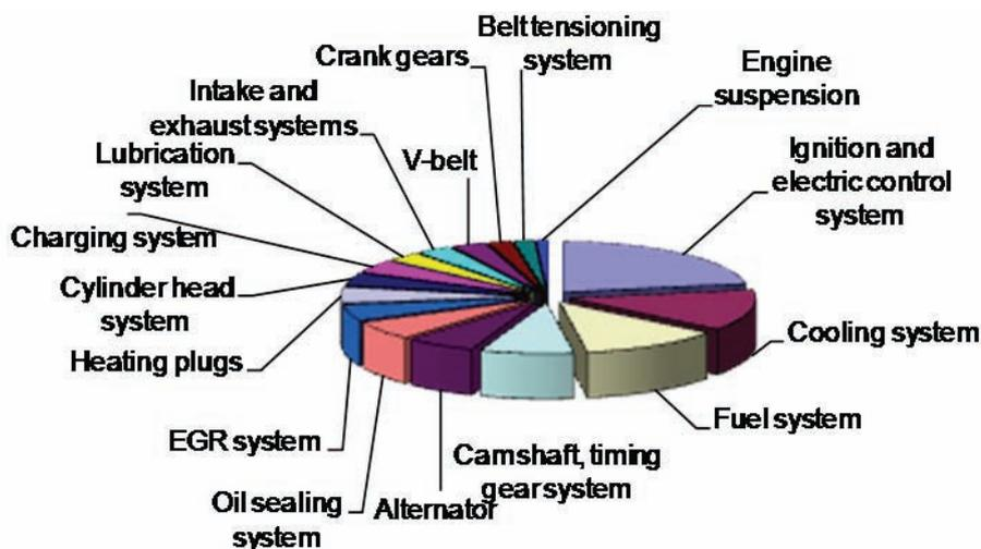
Fig. 4. Structure of engine faults
