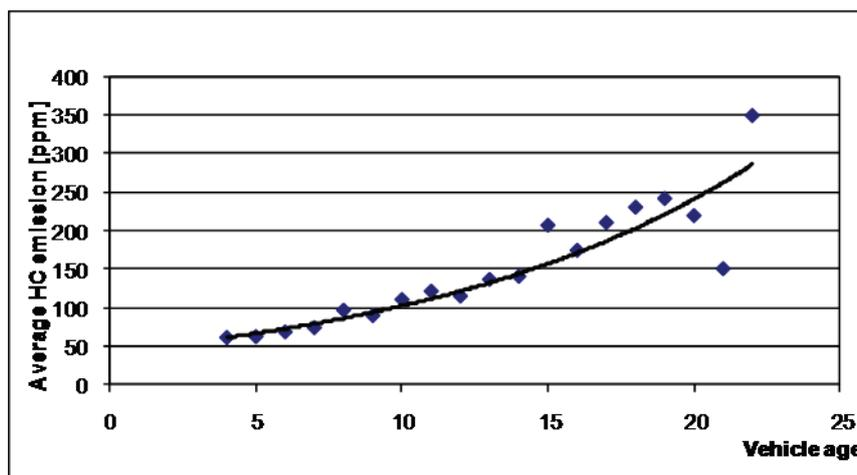
*Fig. 9. Average HC emission for a particular vehicle age (800 rpm)*
