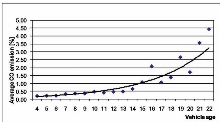
*Fig. 8. Average CO emission for a particular vehicle age (2500 rpm)*
