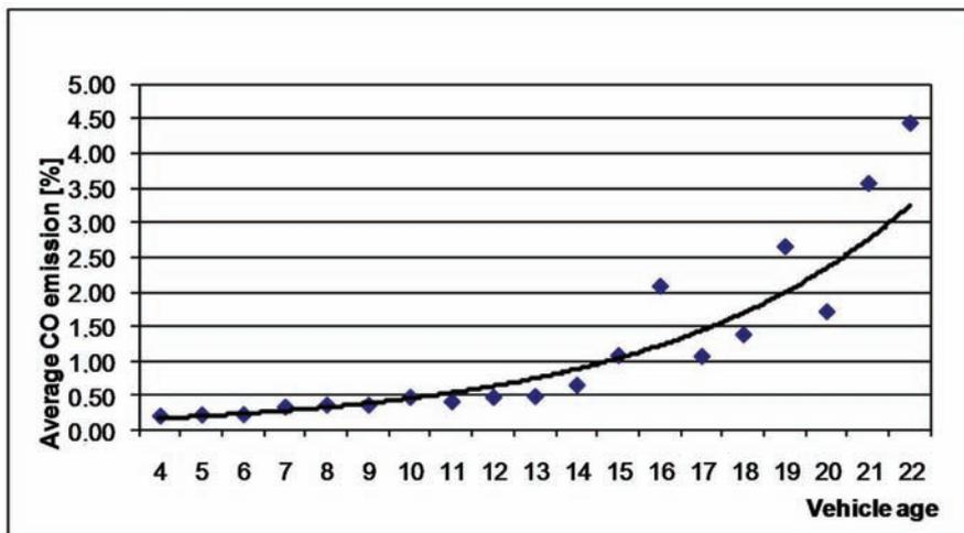
Fig.7. Average CO emission for a particular vehicle age (800 rpm)
