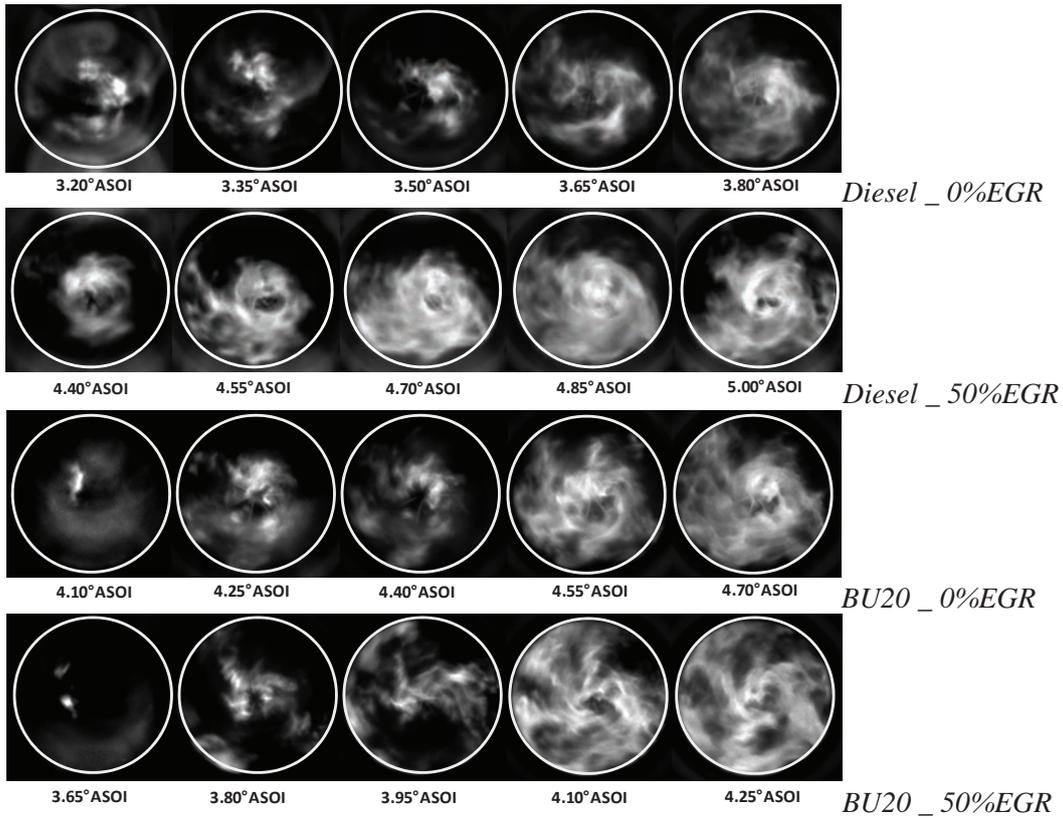
Fig. 5. UV-VIS flame emission for Diesel and BU20, SOI=11 CAD BTDC (0-50%EGR)
