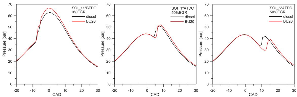
Fig. 1. In-cylinder pressure for diesel and BU20 for selected engine conditions
