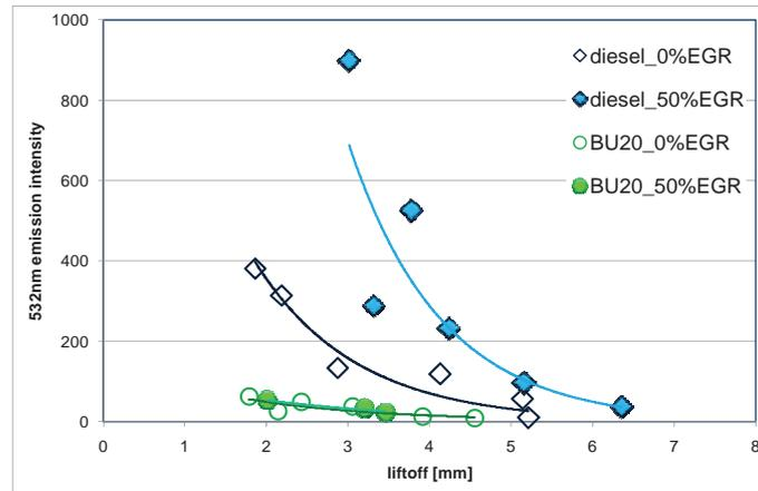
Fig. 8. Integral emission intensity versus the lift-off length measured by filtered data at 532 nm for all the selected operative conditions and fuels
