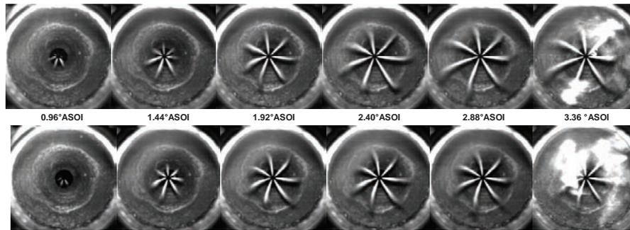
Fig. 4. Cycle resolved spray evolution for diesel fuel at SOI=11 CAD BTDC (up) and 1 CAD ATDC (down) at EGR=0%
