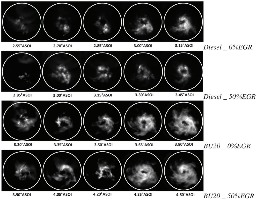
Fig. 6 - UV-VIS flame emission for Diesel and BU20, SOI=3 CAD BTDC (0-50%EGR)
