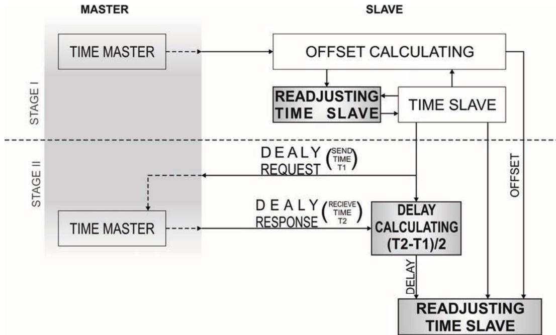
Fig. 2. Example of PTP synchronization
