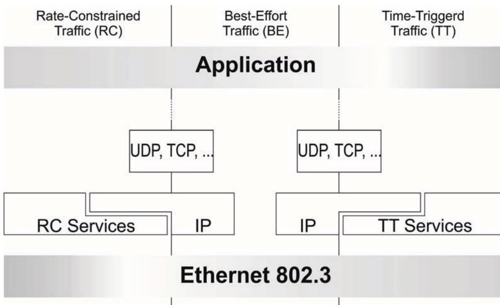
Fig. 6. Relation of TTEthernet to existing communication Standards [16]
