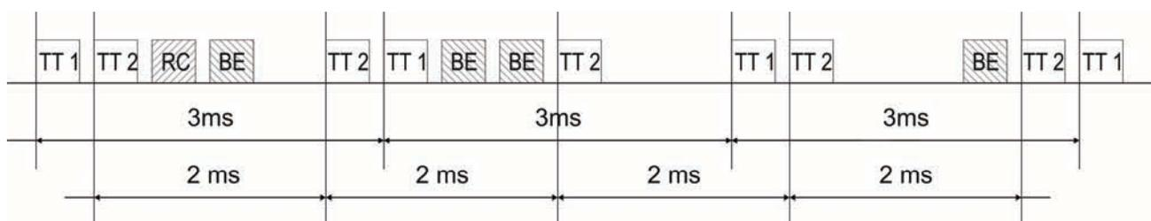
Fig. 5. Partitioning time between TTEthernet messages
