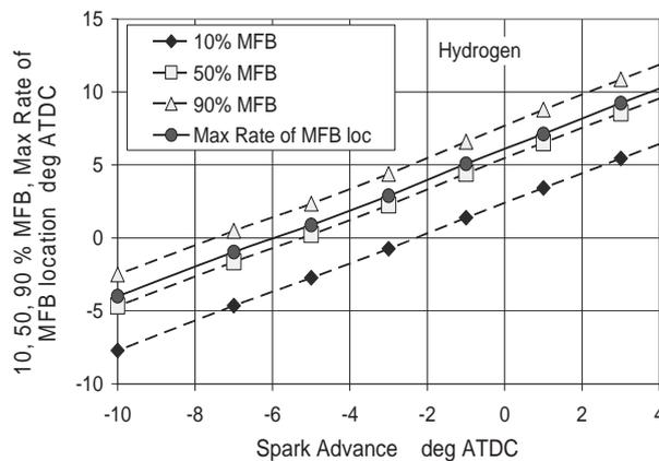
Fig. 3. 10, 50, 90% MFB and maximum rate of MFB locations vs. spark timing for the hydrogen engine with CR = 10
