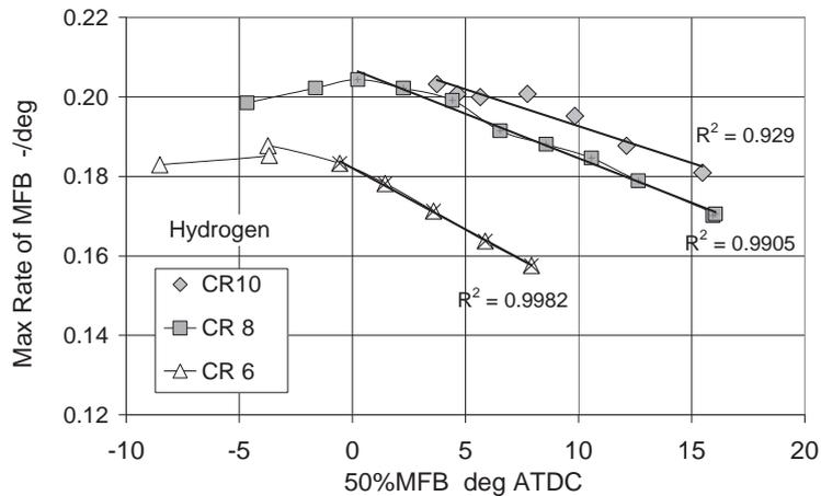
Fig. 5. Maximum rate of MFB against 50% MFB location for the hydrogen fuelled engine at CR=6, 8, 10
