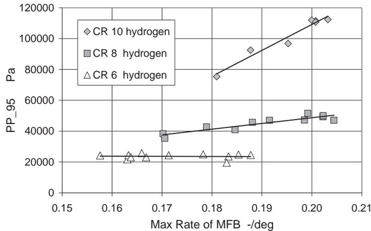
Fig. 6. Knock intensity  $PP_{95}$  vs. maximal rate of MFB for the hydrogen fuelled engine at  $CR=6, 8, 10$
