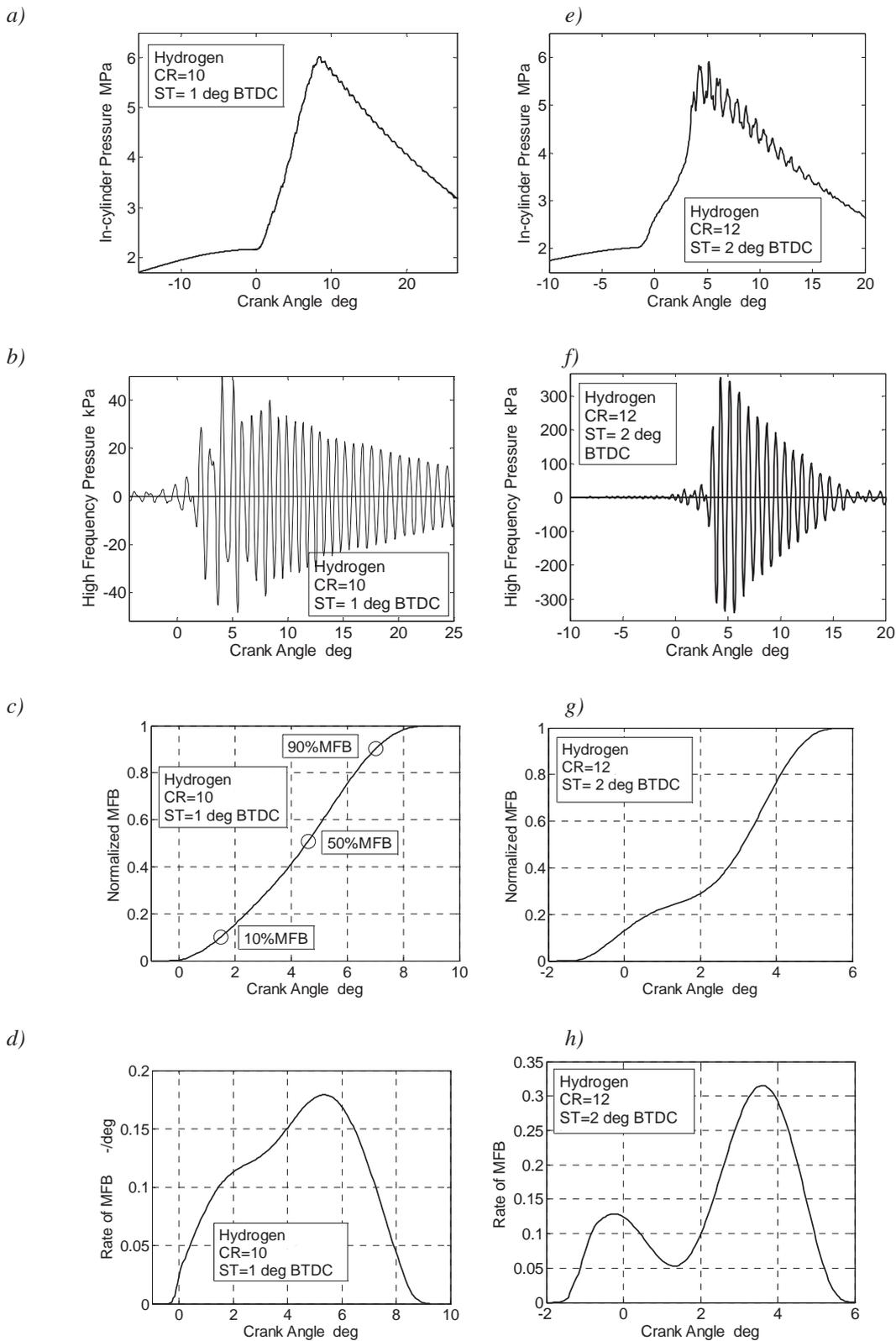
Fig. 1. Combustion events of hydrogen fuelled engine: at light knock (a, b, c, d) and strong knock (e, f, g, h): a, e) in-cylinder combustion pressure, b, f) high frequency pressure component, c, g) MFB profile, d, h) rate of MFB
