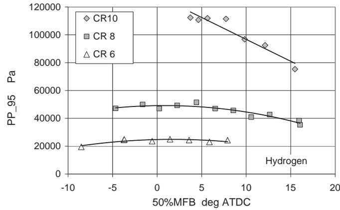
Fig. 4. Knock intensity  $PP_{95}$  vs. 50% MFB location for the hydrogen fuelled engine
