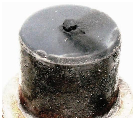
*Fig. 4. View of injector hole pintle nozzle coking field of CFR engine for Cetane number determination (O&GI Cracow)*
