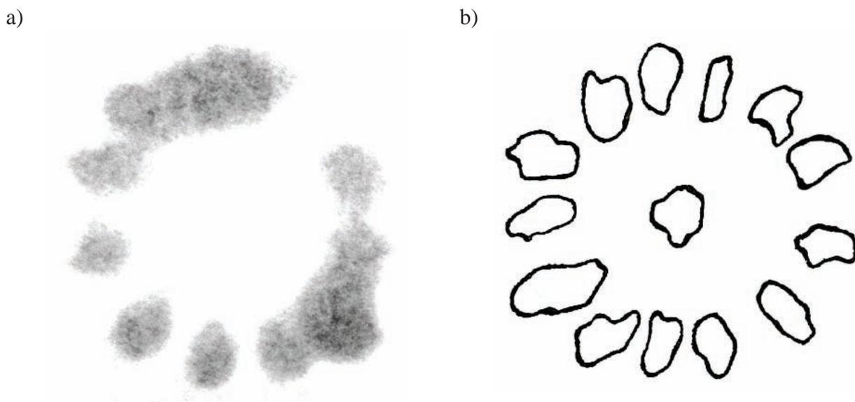
Fig. 7. Comparison of spraying stream fuel distribution through injector of CFR Waukesha test engine after biofuels determinations (a) with standard distribution according to ASTM D 613 (b) – (O&GI Cracow)
