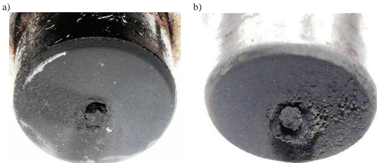
*Fig. 12. The injectors of CFR Waukesha test engine after determinations CN for biofuel B30 (a) and biodiesel B100 (b) – (O&GI Cracow)*
