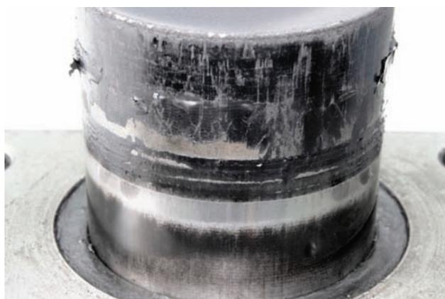
*Fig. 5. Carbon deposit on piston crown and piston skirt of manual setting wheel for change of test engine combustion chamber volume (O&GI Cracow)*
