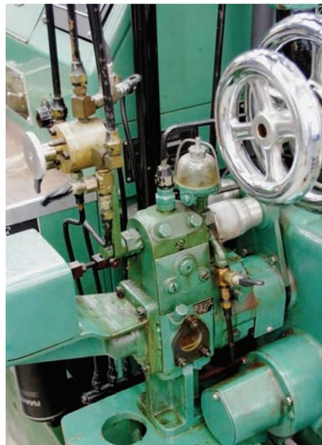
*Fig. 2. Single-assembly fuel injection pump of CFR Waukesha engine for Cetane number determination according to ASTM D 613 (O&GI Cracow)*
