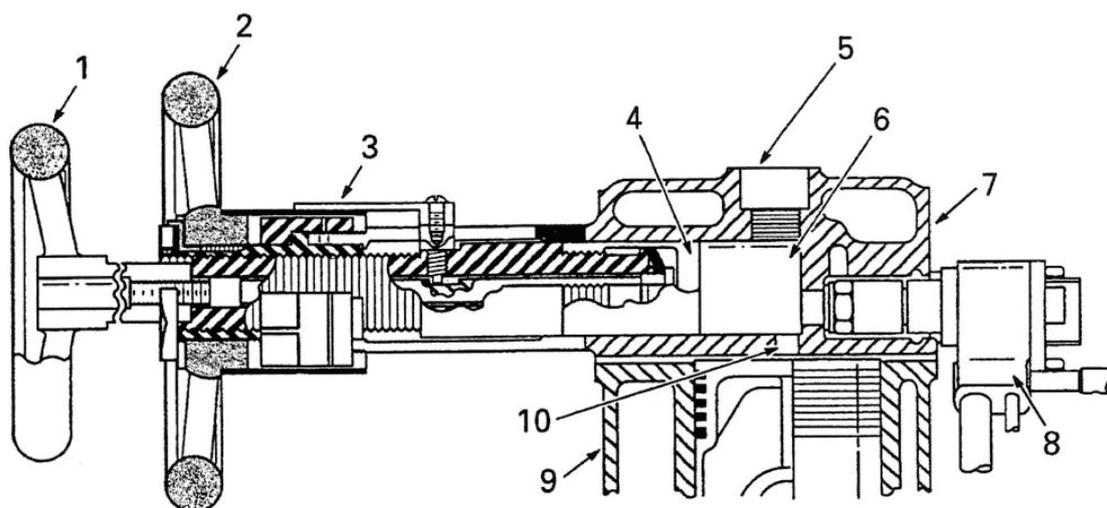
Fig. 3. Review picture engine's combustion chamber for the determination of Waukesha CFR Cetane number and piston assembly of the handwheel is used to change the volume of the combustion chamber: 1- variable compression plug –locking wheel; 2- variable compression plug –handwheel; 3- variable compression plug – micrometer; 4-variable compression plug, 5-combustion pickup hole; 6-precombustion chamber, 7-cylinder head; 8-injector nozzle assembly; 9-cylinder; 10-turbulence passage (ASTM D 613)
