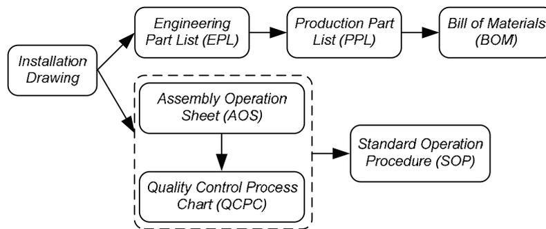
Fig. 2. Engineering processing in utilizing product installation drawing
