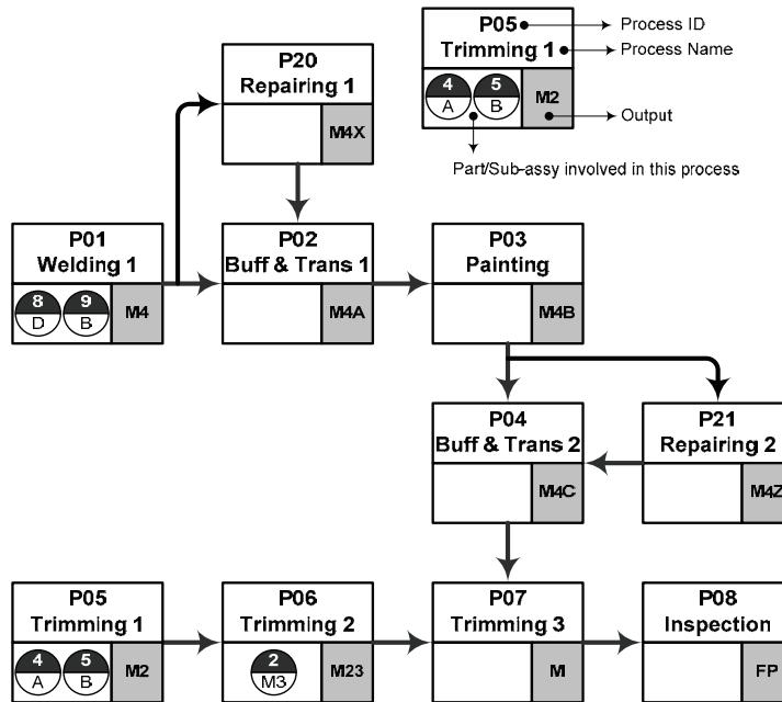
Fig. 4. Model of process which shows sequence of production process
