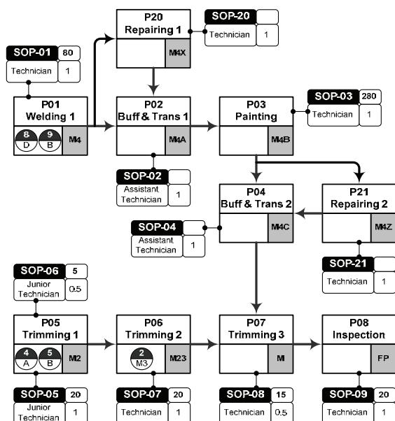
Fig. 5. Relation among SOP model with production process sequences
