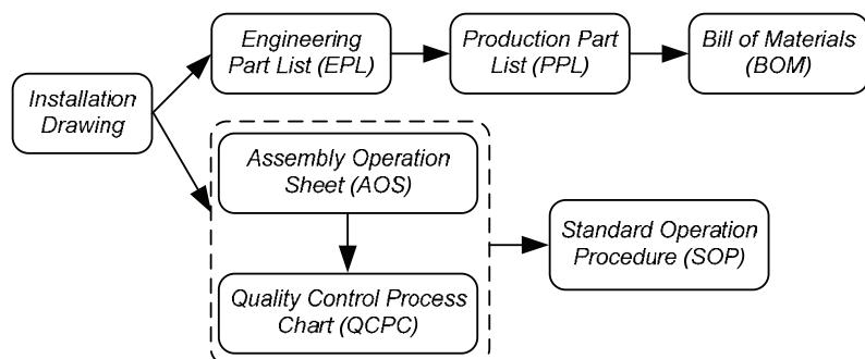
Fig. 2. Engineering processing in utilizing product installation drawing
