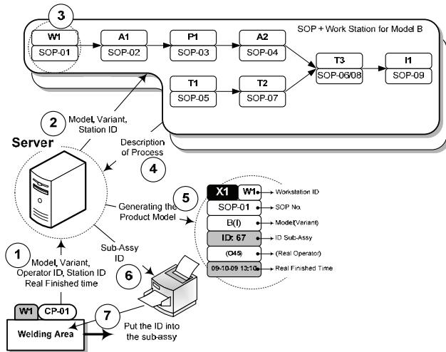
Fig. 9. An initialization mechanism at the product model construction
