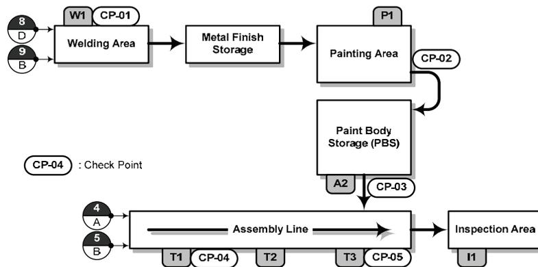
Fig. 8. An example of the monitoring point location design
