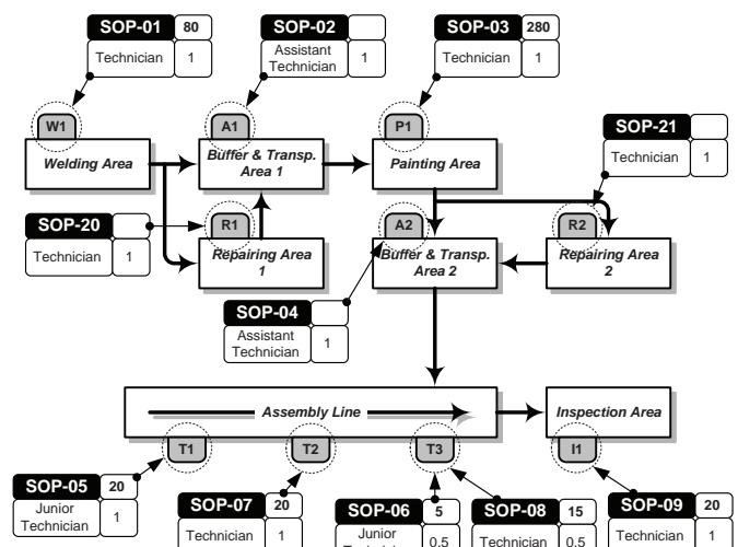
Fig. 6. Mapping of standard operation procedure to a production unit
