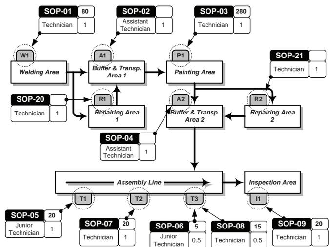
Fig. 5. Relation among SOP model with production process sequences
