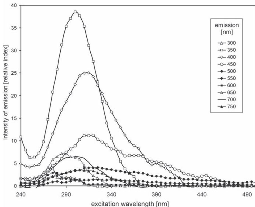
Fig. 2. Excitation spectra for various emission wavelength (for exemplary oil the same as in Fig. 1)
