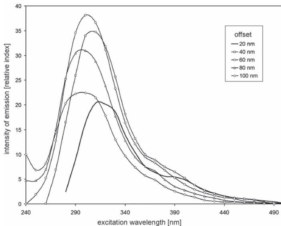
Fig. 3. Synchronous spectra for various offset for exemplary oil (the same as in Fig. 1)
