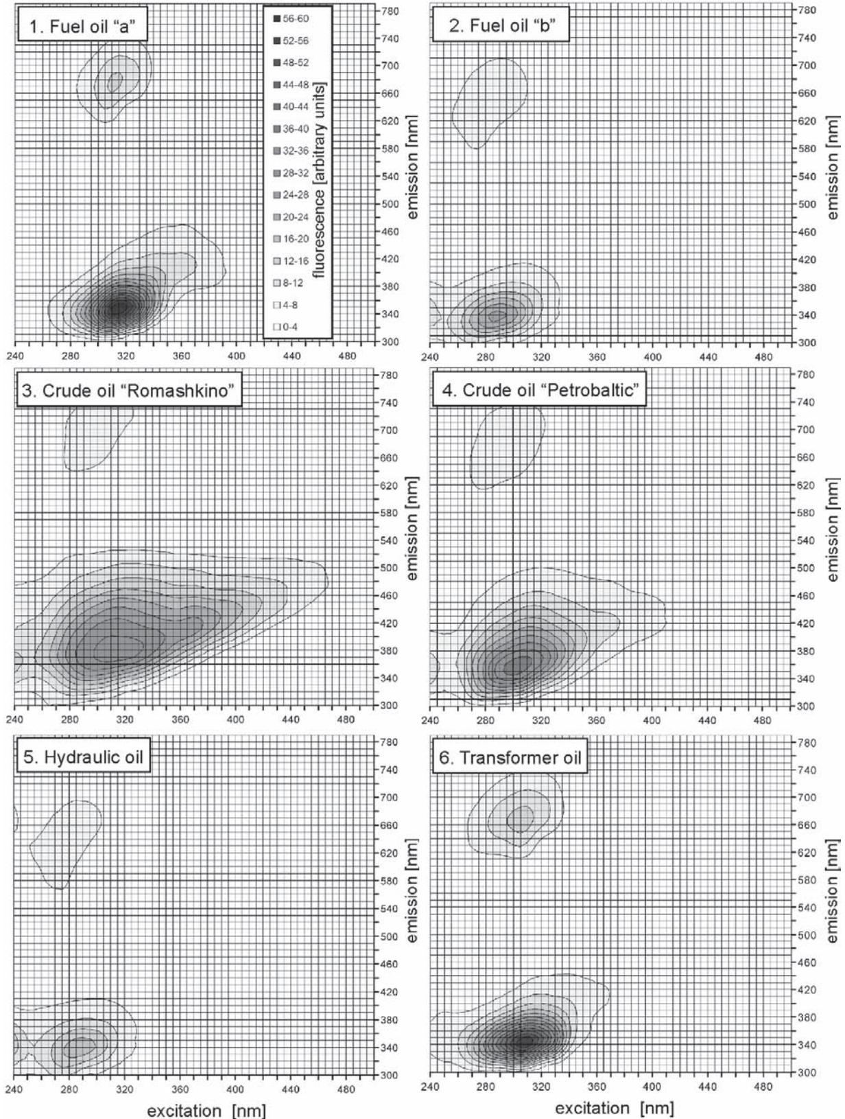
Fig. 4. Total fluorescence spectra for chosen oils
