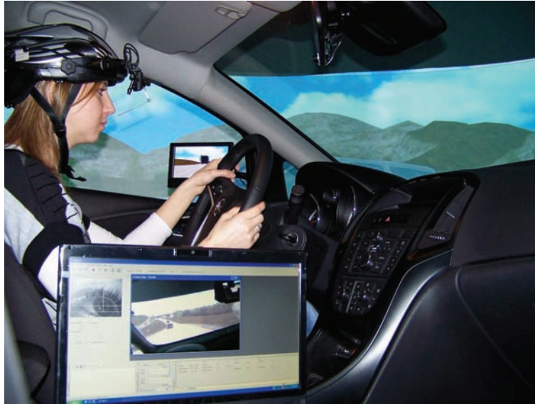
Fig. 3. Use of SMI iView X HED Eyetracker system in passenger car simulator AS1200-6
