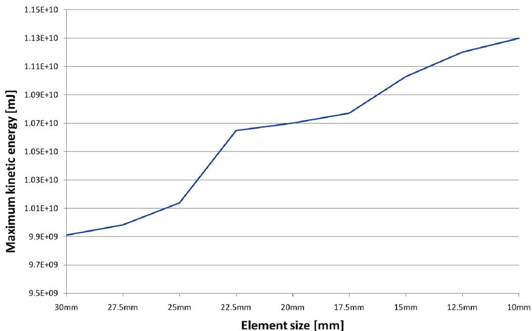
Fig. 6. Maximum Eulerian domain kinetic energy vs. element size
