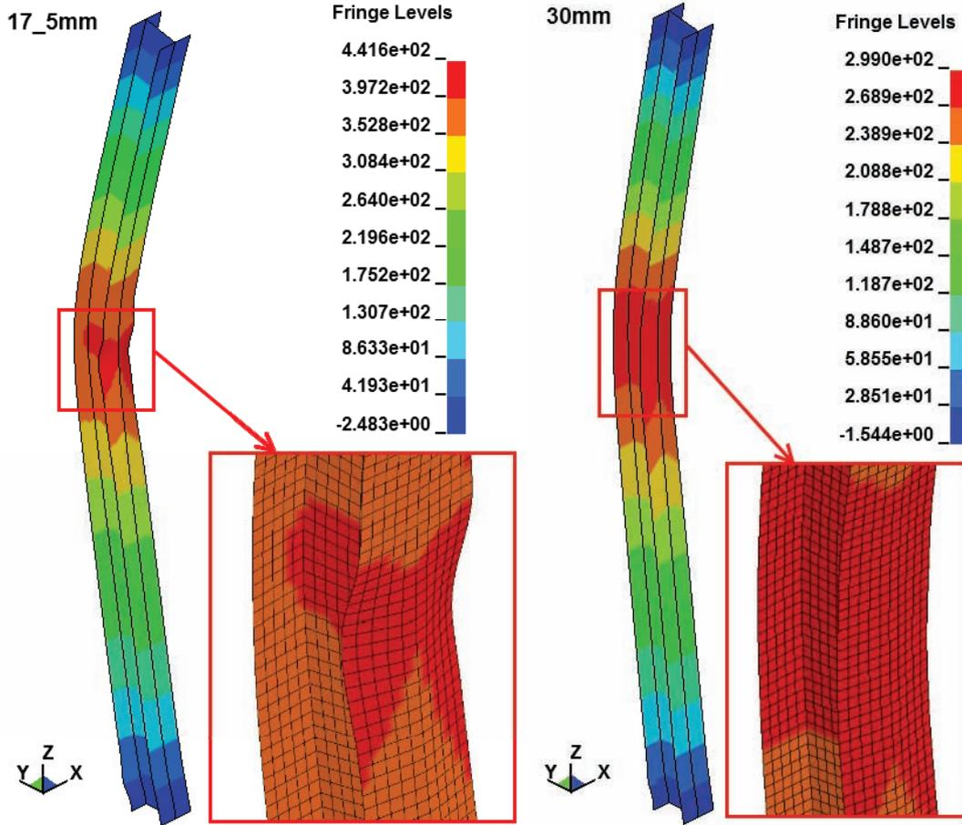
*Fig. 7. Map of Y-displacement [mm]*
