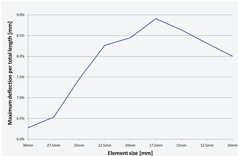
Fig. 5. Maximum column deflection in function of Eulerian mesh element size
