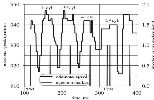
Fig. 12. Rotational speed fluctuation at idle speed with 2-phase injection
