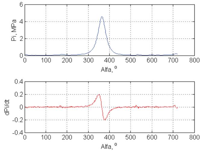
Fig. 7. Cylinder pressure at idle speed with 1-phase injection and malfunction at 4<sup>th</sup> cylinder
