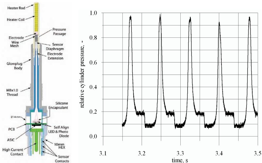
Fig. 4. Cylinder pressure: a) low cost sensor integrated on glow plug [17], b) exemplary pressure course obtained from pressure sensor
