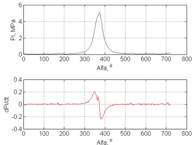
Fig. 8. Cylinder pressure at idle speed with 1- phase injection
