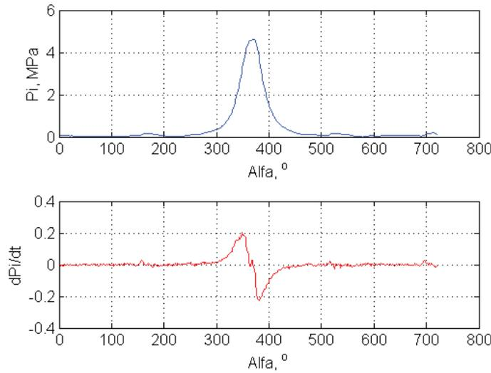
Fig. 9. Pressure at 1<sup>st</sup> cylinder at idle speed with 2-phase injection (modified)
