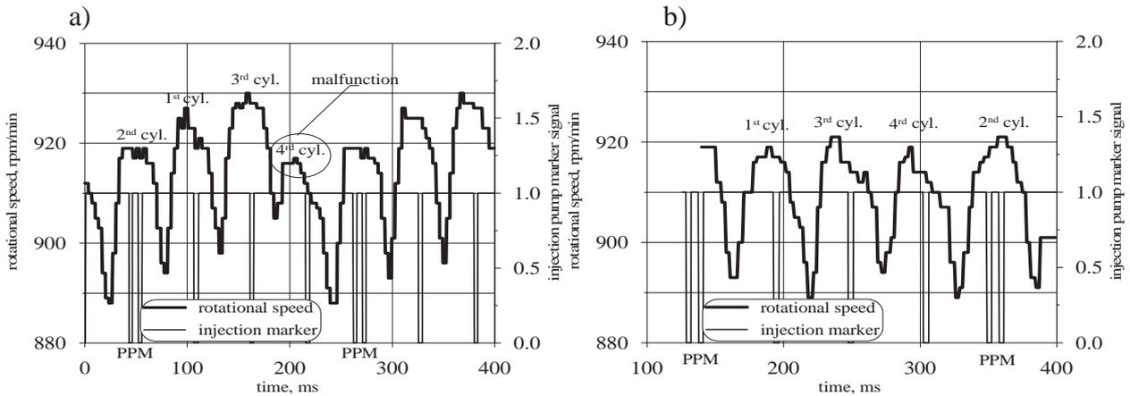
Fig. 11. Rotational speed fluctuation at idle speed with a) 1-phase injection and malfunction at 1st cylinder b) 1 phase and injection correction at 1st and 4rd cylinder
