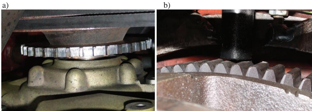
Fig. 6. Engine speed sensors: a) standard-36 tooth, b) high resolution -129 tooth
