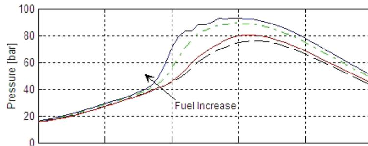
Fig. 2. Influence of fuel injection system control at course of cylinder pressure [4]
