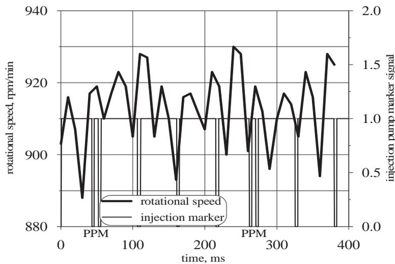
Fig. 10. Rotational speed fluctuation at idle speed with 1-phase injection and malfunction at 1<sup>st</sup> cylinder from standard rotational speed sensor
