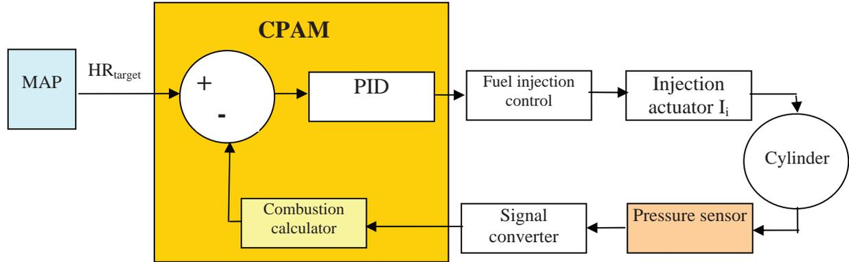
Fig. 5. Schema of injection control with CPAM and cylinder pressure sensor
