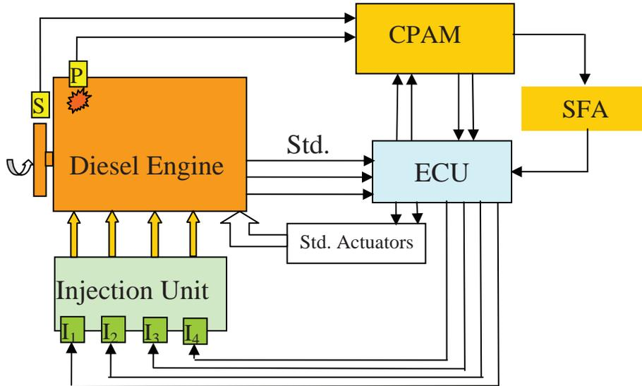
Fig. 3. Conception of Advanced control of injection system with additional analysis modules
