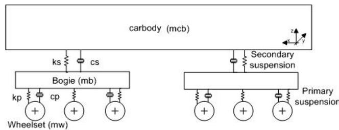
Fig. 2. Multibody model of DH Locomotive
