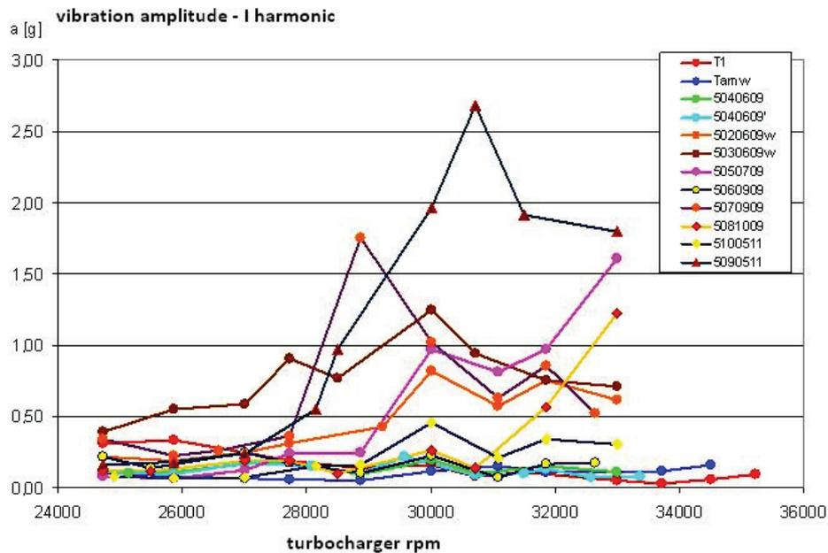
Fig. 13. Vibrations acceleration amplitude – I harmonic measured on turbocharger bearing casing versus turbocharger rpm – twelve turbochargers in different technical conditions tested on the same marine diesel engine stand
