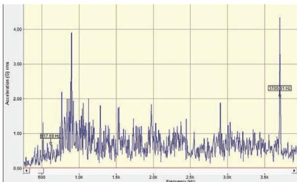
Fig. 5. Acoustic signal spectrum of the turbocharger in frequency range from 0 kHz to 4 kHz
