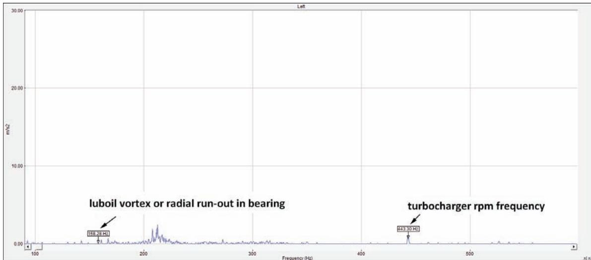
Fig.11. Amplitude of vibrations accelerations in frequency domain for turbocharger in good technical conditions
