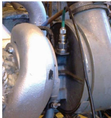
Fig.2a. WSK–Holset 4MD type turbocharger with vibration sensor mounted on the bearing housing
