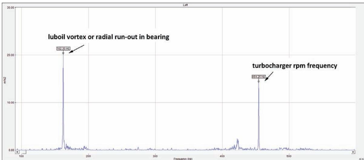
Fig. 12. Amplitude of vibrations accelerations in frequency domain for turbocharger in bad technical conditions
