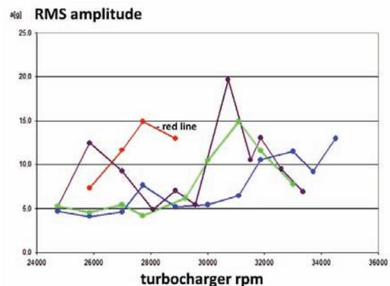
Fig. 8. RMS amplitudes for three turbochargers. Red line – turbocharger in bad technical condition. Blue, violet and green – turbochargers in good technical conditions
