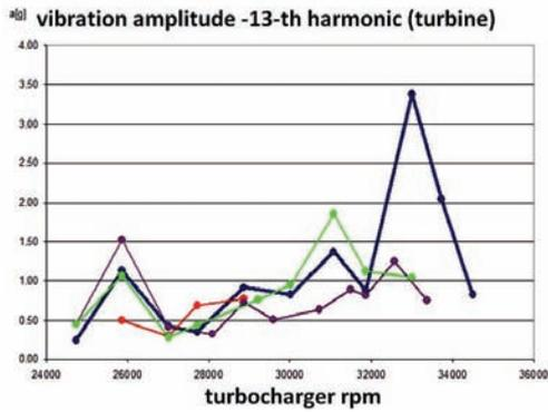
Fig. 9. Value of 13-th harmonic vibrations of accelerations equivalent of turbine blades number
