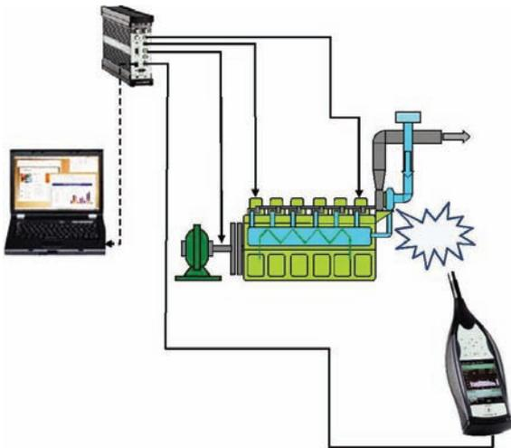
Fig. 2. Acoustic and vibration parameters measuring system configuration on stands of WOLA 57H6Aa and SULZER 6AL20/24 type high-speed diesel engines
