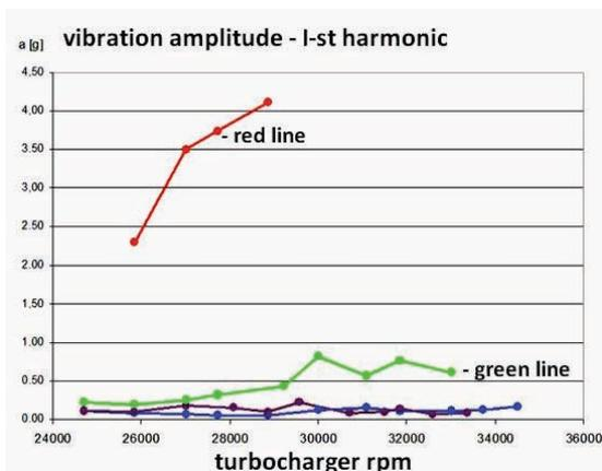
Fig. 7. Vibration acceleration amplitude of first harmonic for three turbochargers. Blue and violet line - turbochargers in good technical condition. Red and green line - turbocharger in bad technical condition (red) and after repair (green)
