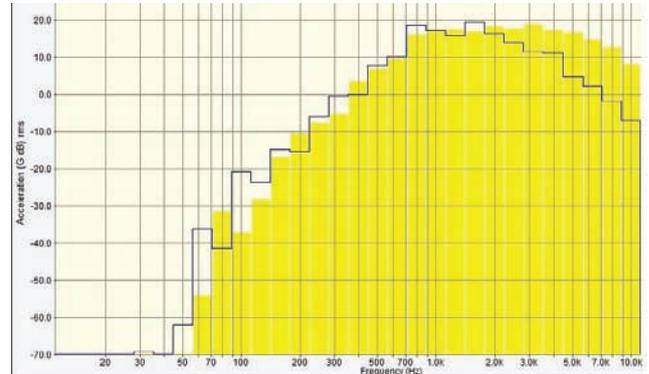
Fig. 4. Acoustic spectrum of turbocharger in octave mode for two different technical conditions – Yellow (grey) – air filter and silencer removed from the turbocharger
