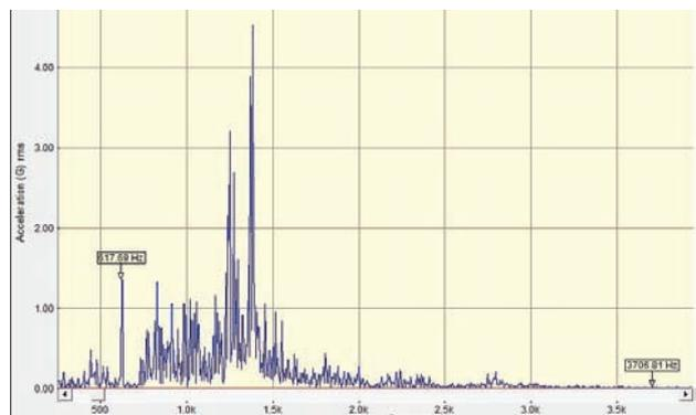
Fig. 6. Vibration signal spectrum of the turbocharger in frequency range from 0 kHz to 4 kHz – magnetic sensor holder
