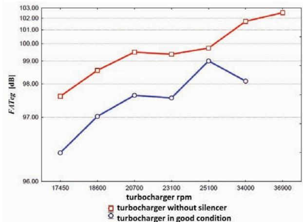
Fig. 3. Sound intensity level of turbocharger in two different technical conditions – blue (lower) – turbocharger in proper technical condition, - red (upper) – air filter and silencer removed from the turbocharger
