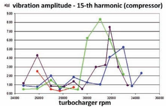
Fig. 10. Value of 15-th harmonic vibrations of accelerations equivalent of compressor blades number
