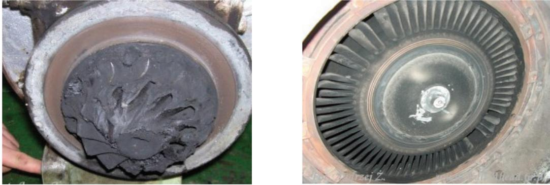
Fig. 1. Examples of radial-flow rotor turbine overgrown by carbon soot (left) and axial-flow rotor turbine without turbine blades (right) [www.ful-ahead.net]
