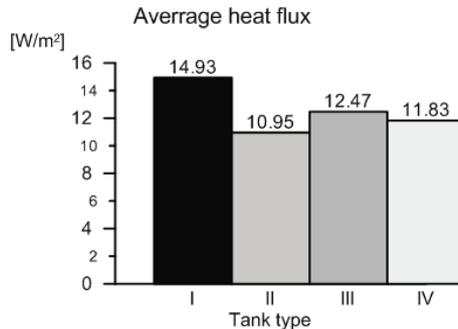
Fig. 9. Comparison of the average heat fluxes of the different tank types
