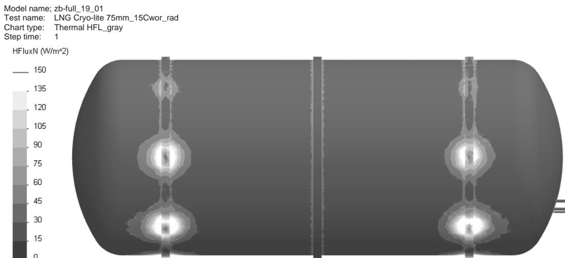
Fig. 3. Heat flux on outer surface of container tank type I
