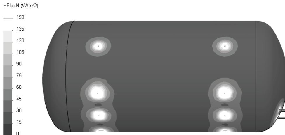
Fig. 6. Heat flux on outer surface of stationery tank type IV
