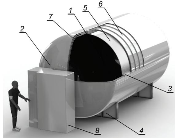
Fig. 2. Model of the mobile LNG, tank type III and IV: 1 – inner tank, 2 – outer tank, 3 – inner supports made of plastic materials, 4 – outer supports, 5 – insulation, 6 – radiation shields, 7 – the vacuum, 8 – fittings
