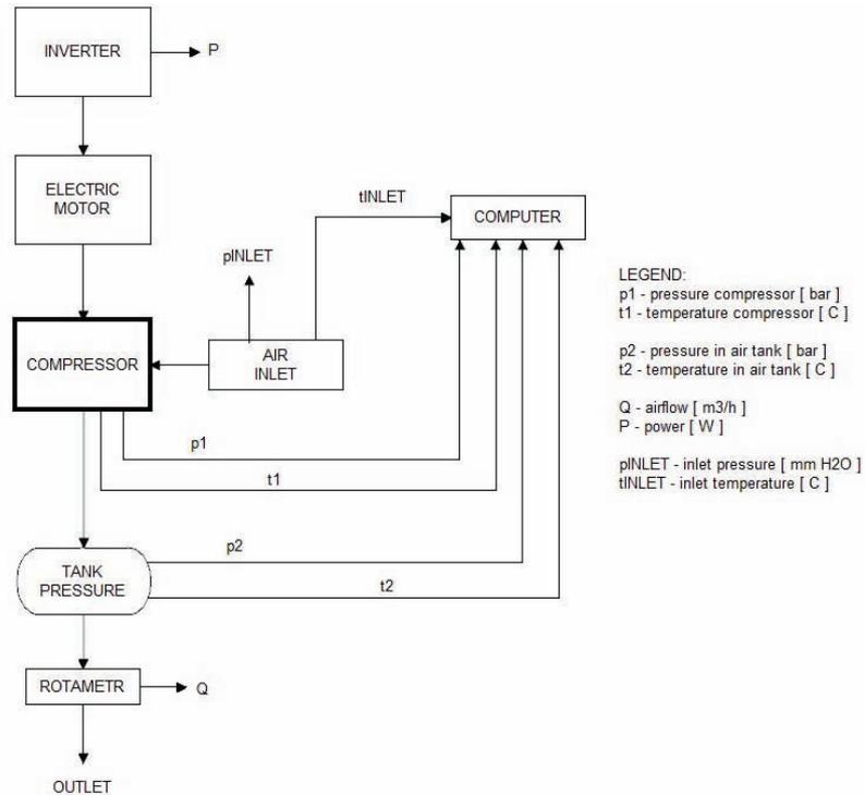
Fig.1. Block diagram of measuring system and test stand built for compressor testing
