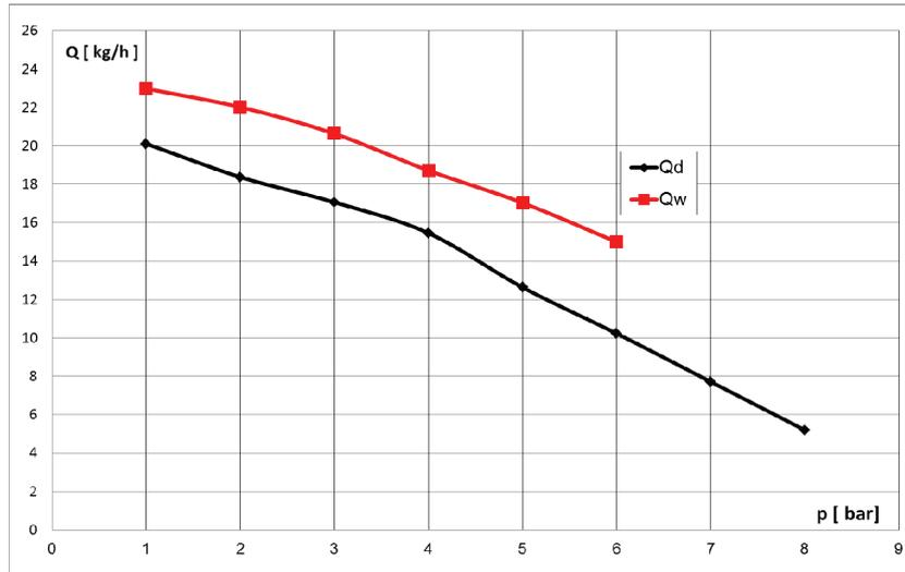
Fig. 4. Inlet ( $Q_d$ ) and outlet ( $Q_w$ ) air flow for engine speed = 970 rpm (PET seal)
