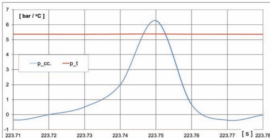
Fig. 8. Air pressure curve in compression chamber at tank pressure of 5,3 bar (zoomed fragment of graph showed)
