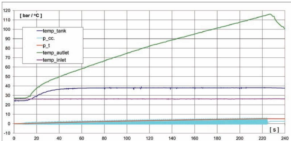
Fig. 7. Variation of pressure and temperature during compressor operation in 0 to 5 bar output pressure range (Temp\_tank – air temperature in tank, p\_cc. - air pressure in compression chamber, p\_t – air pressure in tank, temp\_outlet – air temperature at compressor outlet, temp\_inlet – air temperature at compressor inlet)
