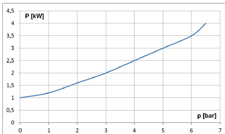
Fig. 10. Compressor power requirement
