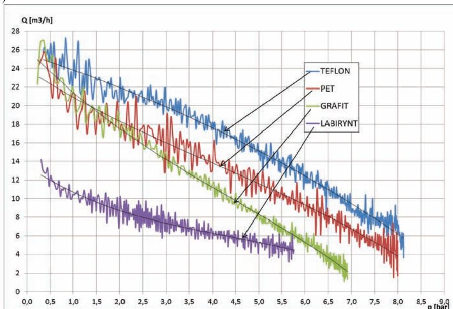
Fig. 9. Comparison of compression rate of blade-type piston compressor for different seal versions
