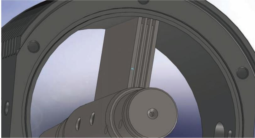
Fig. 6. The 3D-view of localization of labyrinth seals
