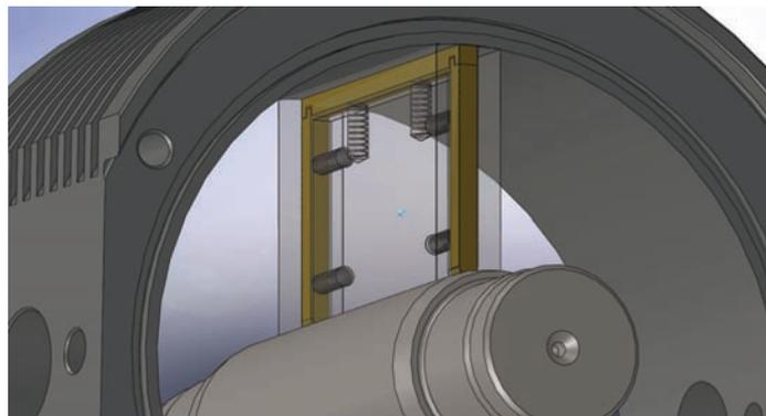
Fig. 3. The 3D-view of localization of contact seals
