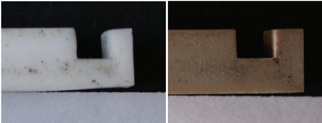
Fig. 5. Deformation of 0.65 mm PTFE seal (left) and 0.35 mm PTE seal (right)
