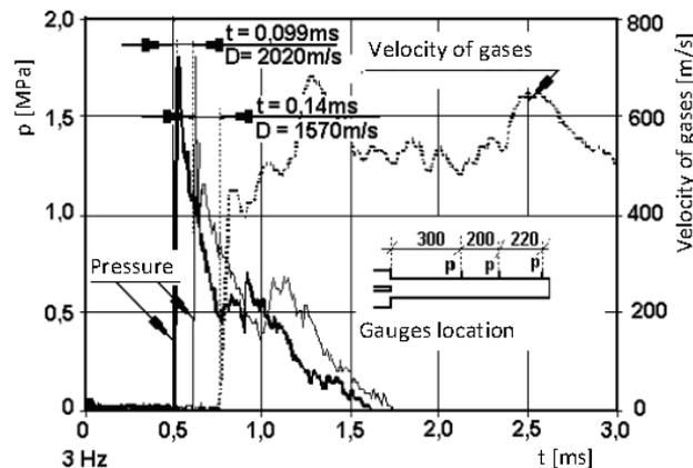
Fig. 4. Pressure and velocity of gas course for the test with frequency equal to 3 Hz
