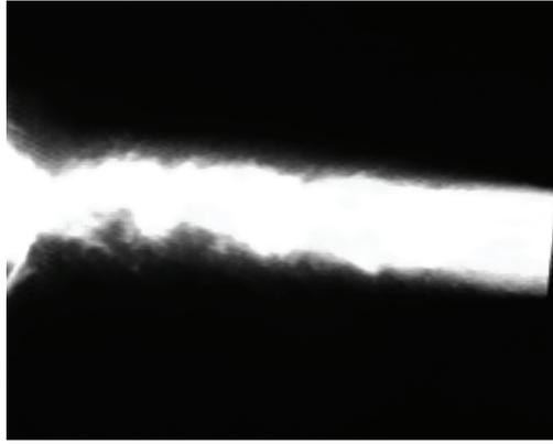
Fig. 7.  $Cr_3C_2+NiCr$  particles jet registered by fast camera. 40 000 f/s, shutter 1. 85  $\mu s$
