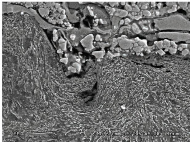
Fig. 8 Structure of WC/Co 83/17 coating on St45 steel substrate
