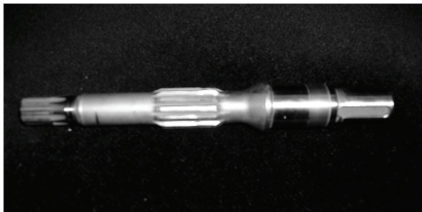
Fig. .11. View of car half-shaft after detonation coating production and grinding.
