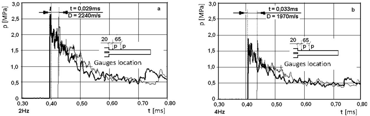
Fig. 2. Influence of the frequency on the pressure and detonation wave velocity, length of the barrel 710 mm: a – frequency 2 Hz; b – frequency 4 Hz
