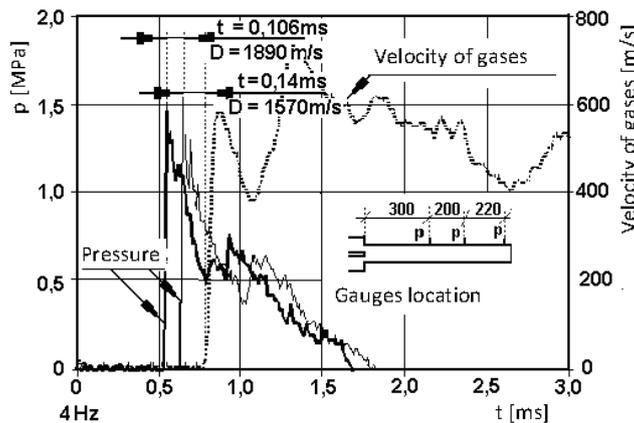
Fig. 3. Pressure and velocity of gas course for the test with frequency equal to 4 Hz
