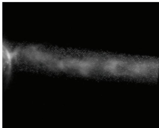
Fig. 6. WC/Co particles jet registered by fast camera. 40 000 f/s, shutter 1. 85  $\mu\text{s}$
