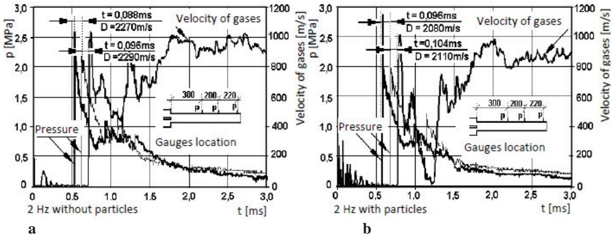
Fig. 5. Pressures and velocity of gases courses for frequency equal to 2 Hz: a – parameters of detonation products; b – parameters of two-phase flow of detonation products and NiCrBSi particles
