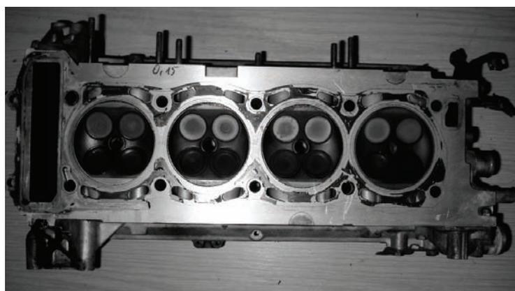
*Fig. 11. Surface of engine head intended for regeneration*
