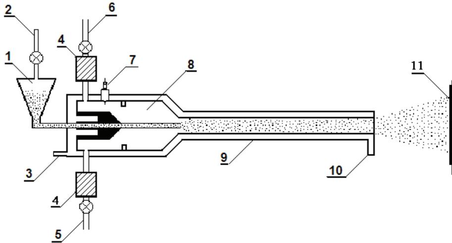
Fig. 1. Scheme of valve-less detonation gun: 1 – coatings particles container; 2 – nitrogen; 3,10 – cooling system; 4 – safety valves; 5 propane-butane; 6 – oxygen; 7 – ignition system; 8 – detonation chamber, 9 – barrel, 11 – substrate
