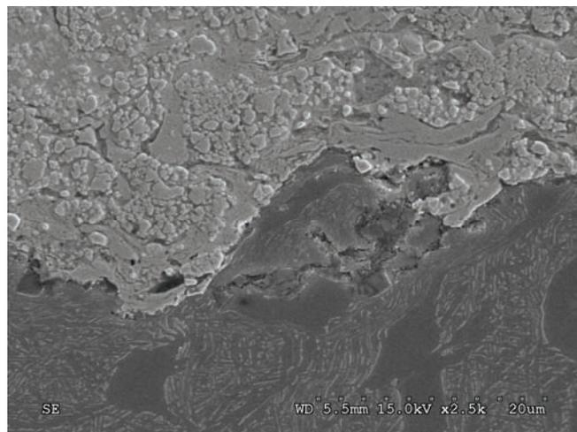
Fig. 9 Structure of WC/Co 83/17 coating on WT3 titanium substrate
