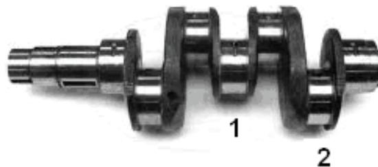
*Fig. 10. View of crankshaft with coatings produced on two pivots: 1 – main pivot, 2 – crank pivot*
