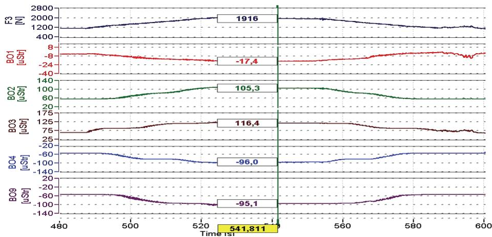
Fig. 6. Captured signals during the experiment. Complex bending and torque load case [4]
