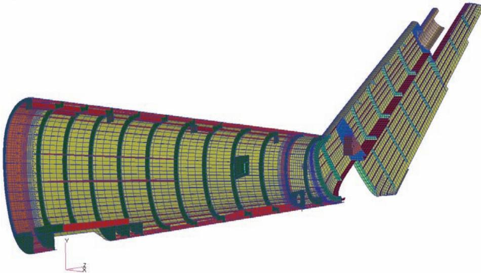
Fig. 1. Global FEM model of the tail boom with vertical stabilizer of the Mi-24 helicopter (right side) [5]
