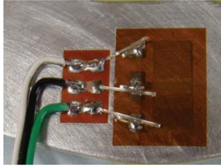
Fig. 3. An example of strain gauge used in analysis
