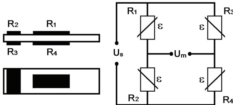
Fig. 4. Strain gauge placement and electrical scheme [6]
