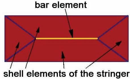
Fig. 5. Numerical strain gauge used in the model
