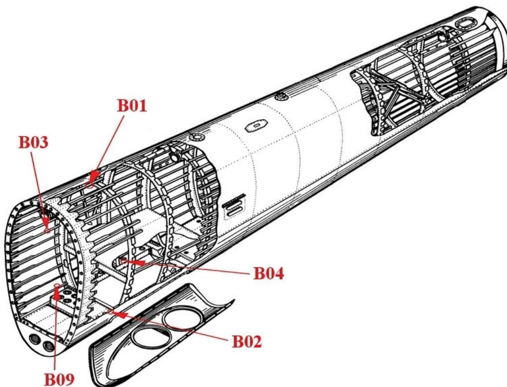
Fig. 2. Localization of the measurement points [2]
