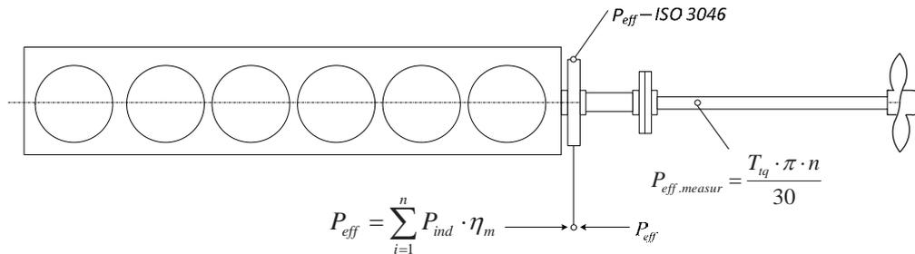
Fig. 1. Main engine shaft power estimation
