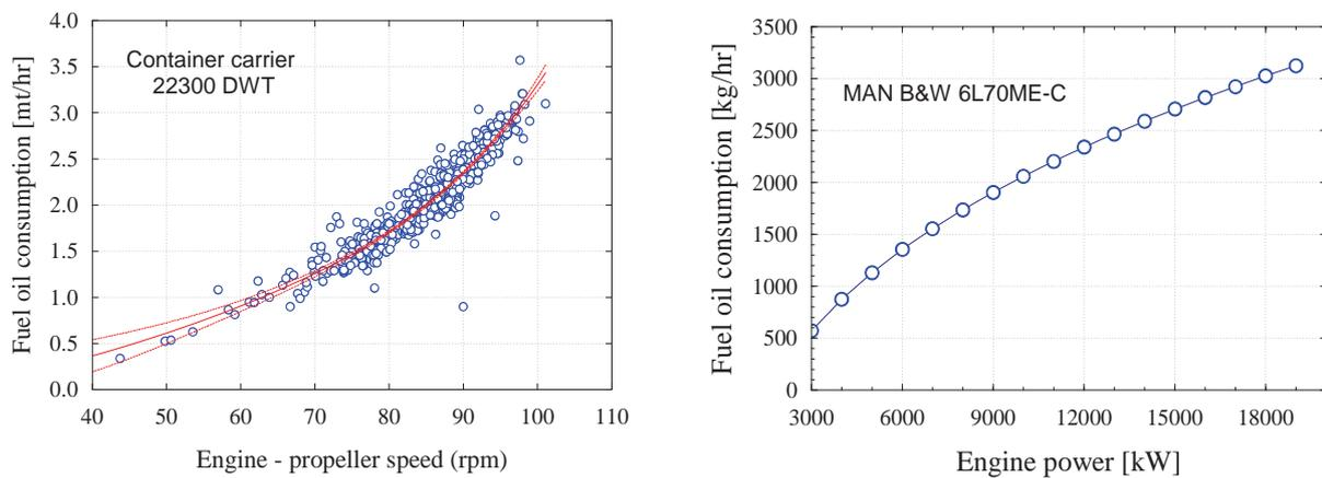
Fig. 6. Fuel oil consumption group and averaged curve for propulsion unit in moderate weather conditions
