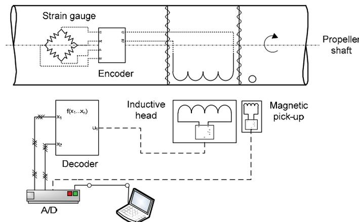
Fig. 2. The main engine shaft power measurement setup
