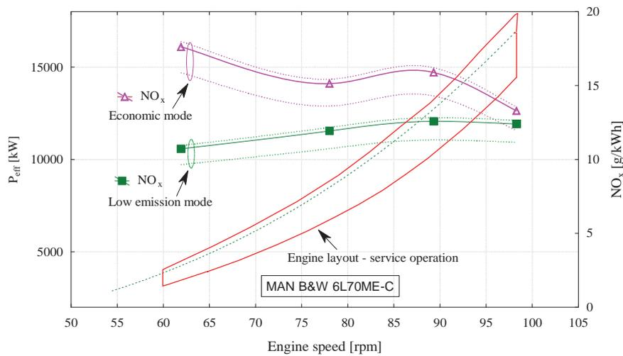
Fig. 8. Example of main engine area operation influenced by weather conditions
