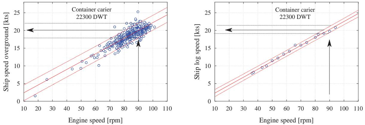
Fig. 7. The ship speed estimated from measured engine – propeller rotational speed
