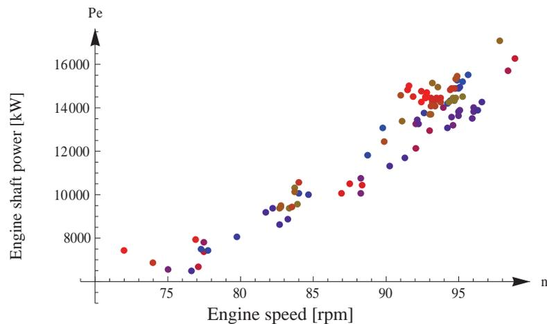
Fig. 3. Examples of main engine shaft power in different conditions
