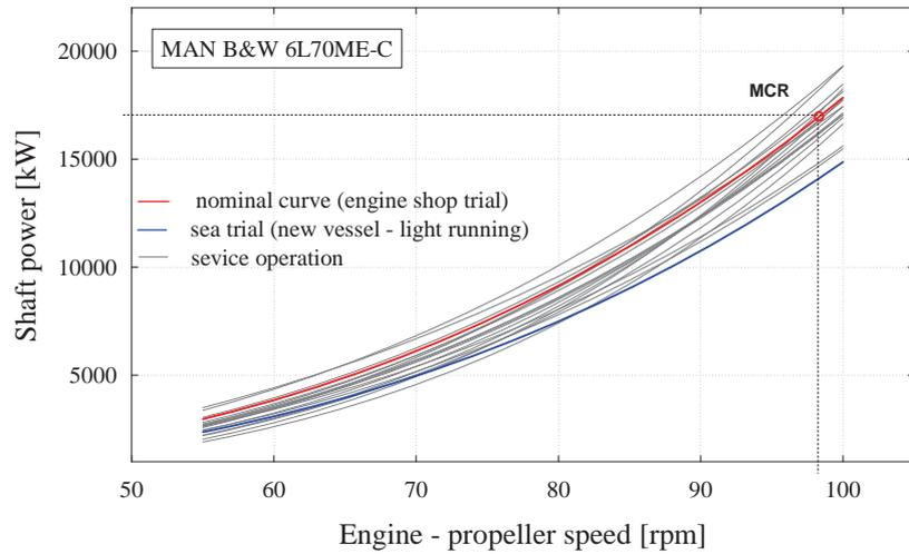
Fig. 5. Example of main engine service operation influenced by weather conditions
