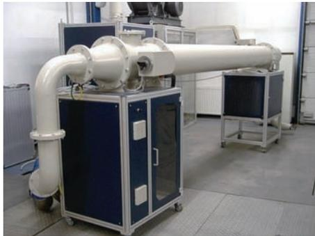
Fig. 7. Dilution exhaust gases device
