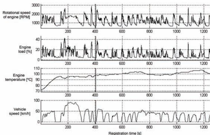
Fig. 2. Vehicle performance record during FTP75 test on chassis dynamometer, implementation of oxygen sensor monitor marked with vertical line, RPM, engine loading [%], engine temperature [ $^{\circ}$ C], speed [km/h]
