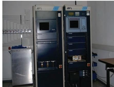
Fig. 8. Exhaust gases analyzers
