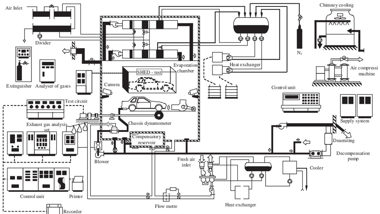
Fig. 6. Scheme of chassis dynamometers stand
