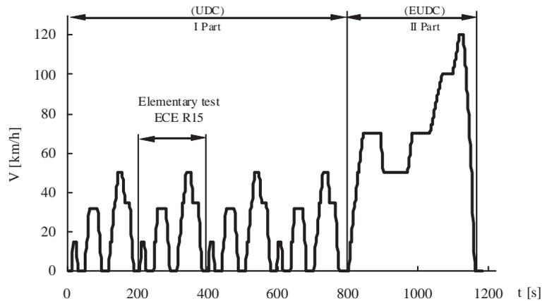
Fig. 3. NEDC (UDC + EUDC) driving test
