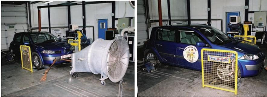
Fig. 4. Chassis dynamometer stands
