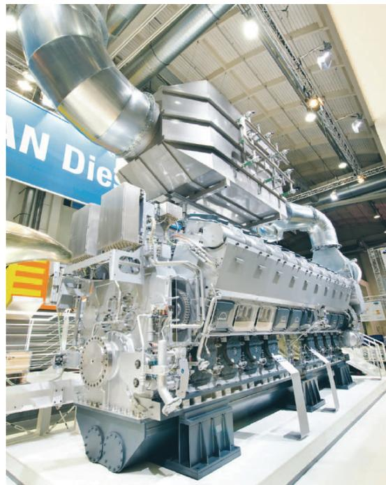
Fig. 8. The 32/44CR engine with SCR pictured at MAN Diesel & Turbo's stand at the SMM Trade exhibition in Hamburg [12]. The engine cracks IMO Tier 3
