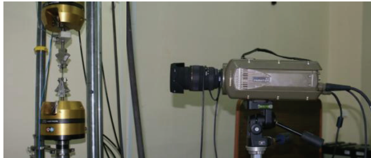
Fig. 1. High-speed camera Phantom V12 and strength machine Instron 8802
