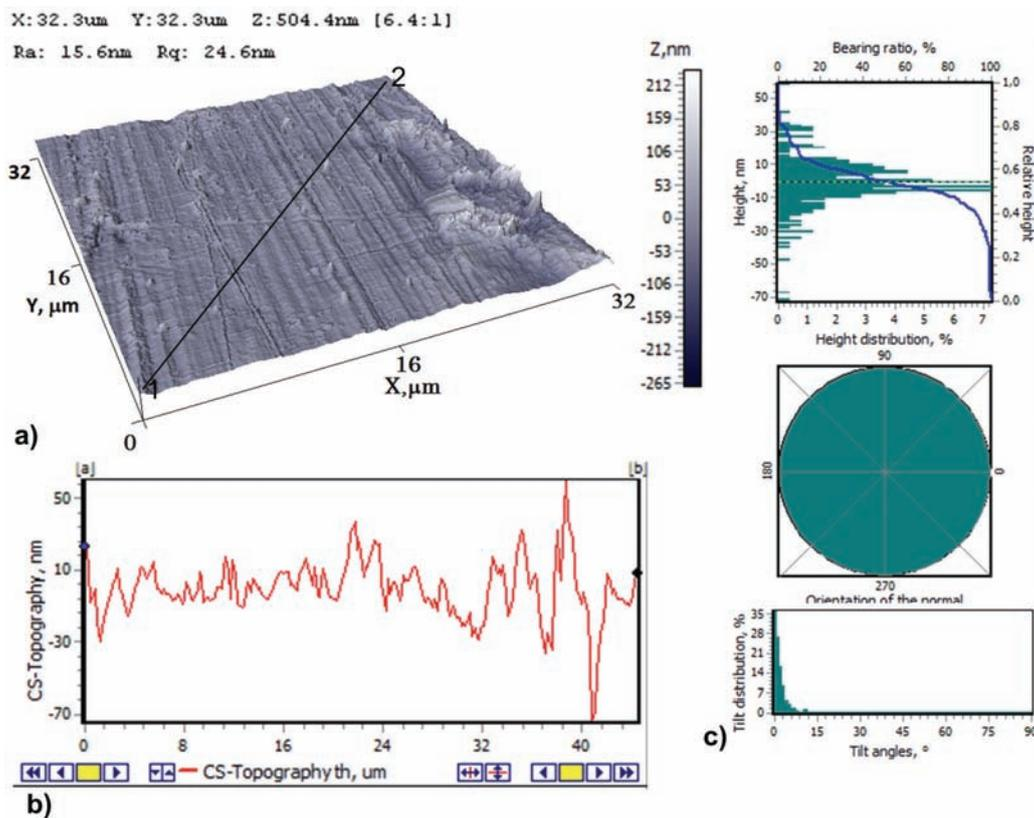
Fig. 7. Surface topography of slide journal micro-bearing sleeve from HDD Seagate Barracuda ST380815AS: a) 3D view, b) cross-section 1-2, c) roughness height distribution, tilts orientation, tilts angles distribution
