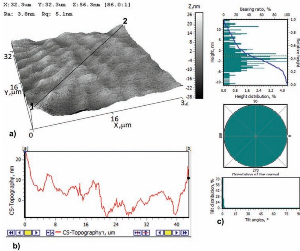
Fig. 6. Surface topography of slide journal micro-bearing sleeve from 2.5" HDD Samsung HM 160 HI: a) 3D view, b) cross-section 1-2, c) roughness height distribution, tilts orientation, tilts angles distribution
