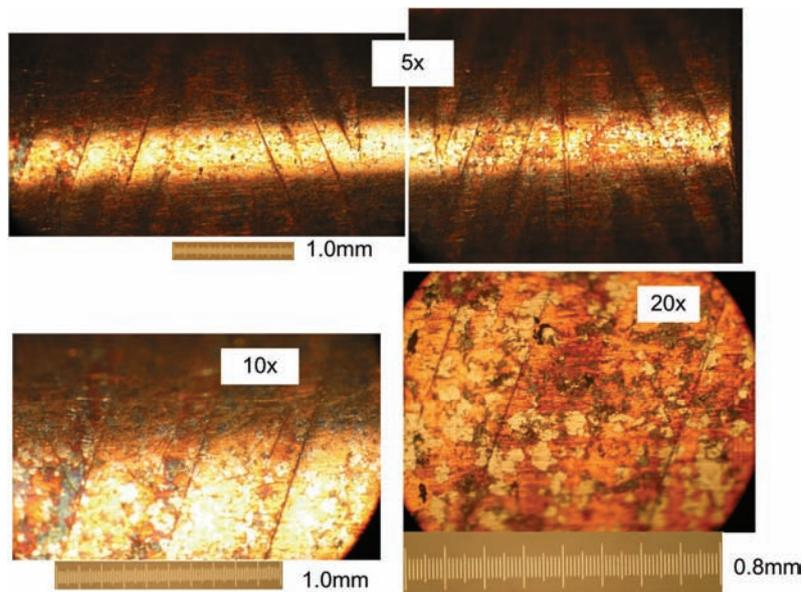
Fig. 3. Bearing sleeve surface with micro-grooves - bearing from 3.5" HDD Seagate Barracuda ST380815AS
