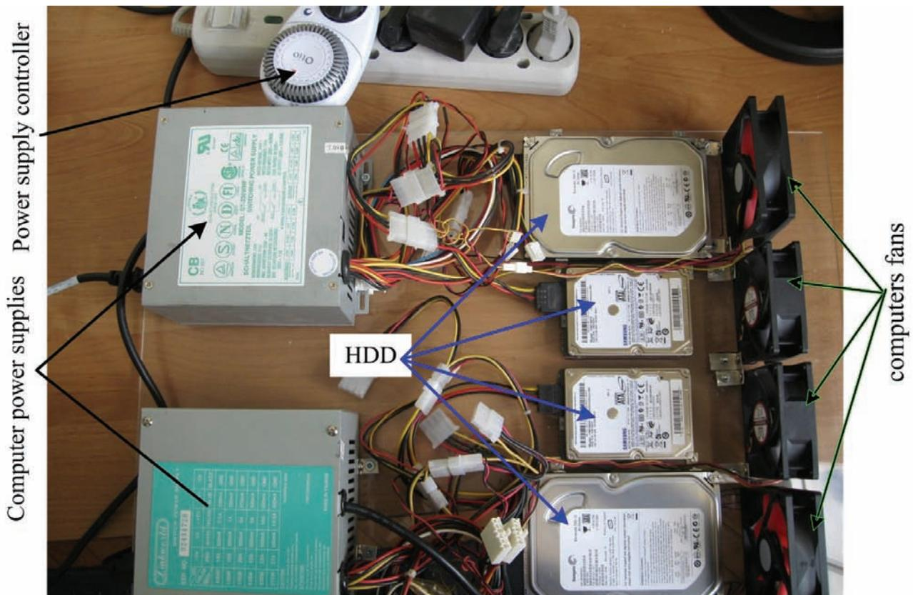
Fig. 1. Working sets of computers hard disk drives and fans
