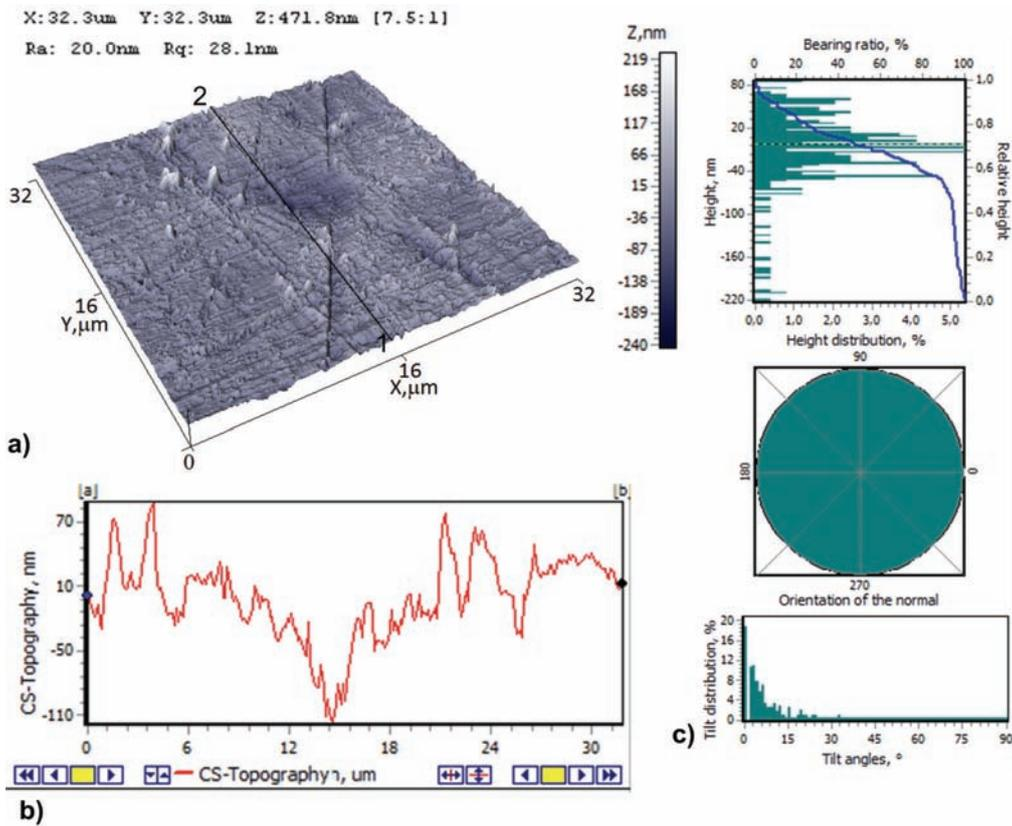
Fig. 9. Surface topography of slide journal micro-bearing sleeve from Xilence Case fan: a) 3D view, b) cross-section 1-2, c) roughness height distribution, tilts orientation, tilts angles distribution
