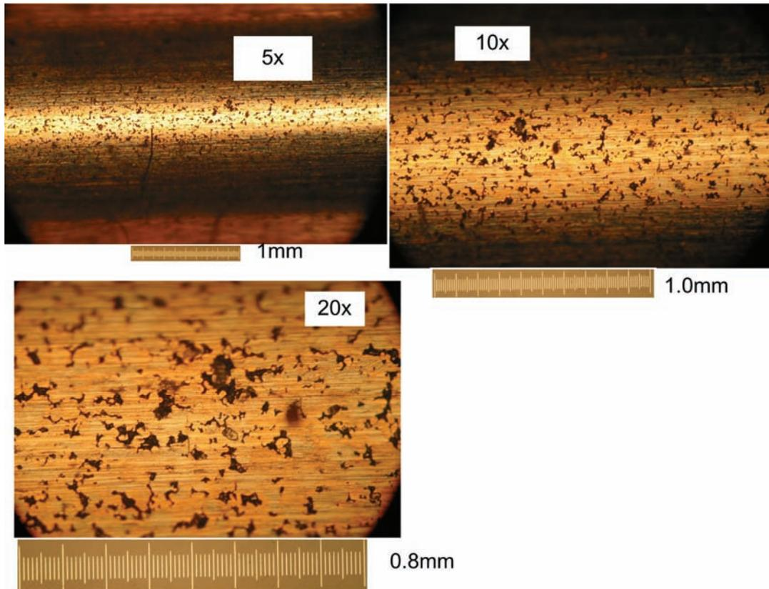
*Fig. 5. Bearing sleeve porous surface - bearing from Xilence Case Fan 92mm*
