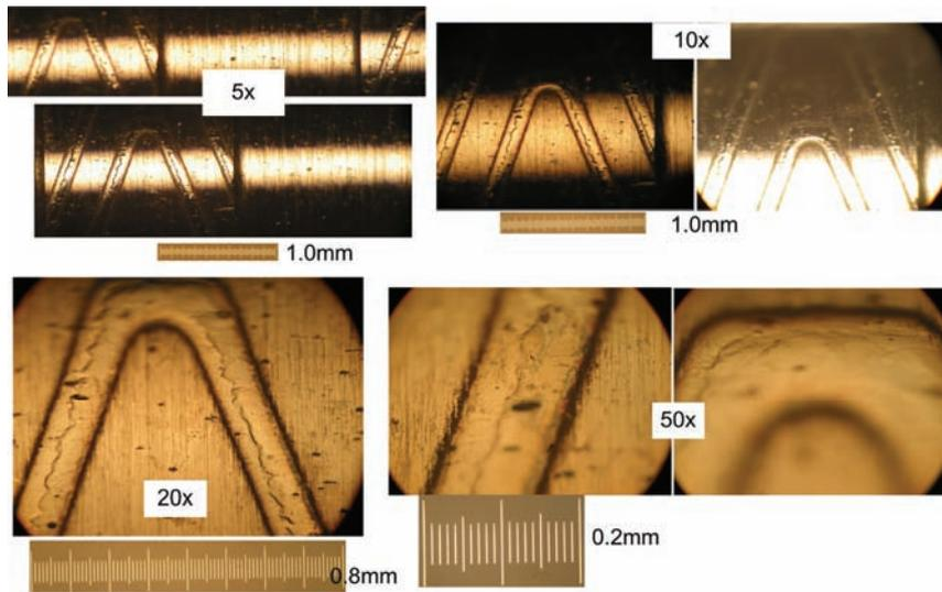
Fig. 2. Bearing sleeve surface with micro-grooves - bearing from 2.5" HDD Samsung HM 160 HI
