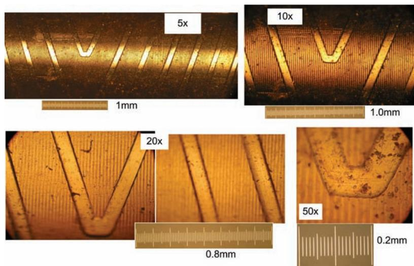
Fig. 4. Bearing sleeve's surface with micro-grooves - bearing from Kama Flow SP0825FDB12H
