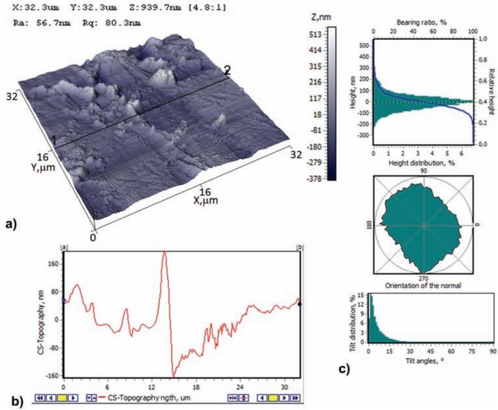
Fig. 8. Surface topography of slide journal micro-bearing sleeve from Kama Flow SP0825FDB12H fan: a) 3D view, b) cross-section 1-2, c) roughness height distribution, tilts orientation, tilts angles distribution
